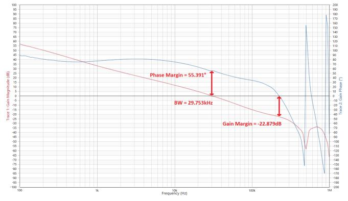
Figure 5-5. Frequency Response IOUT = 6A
