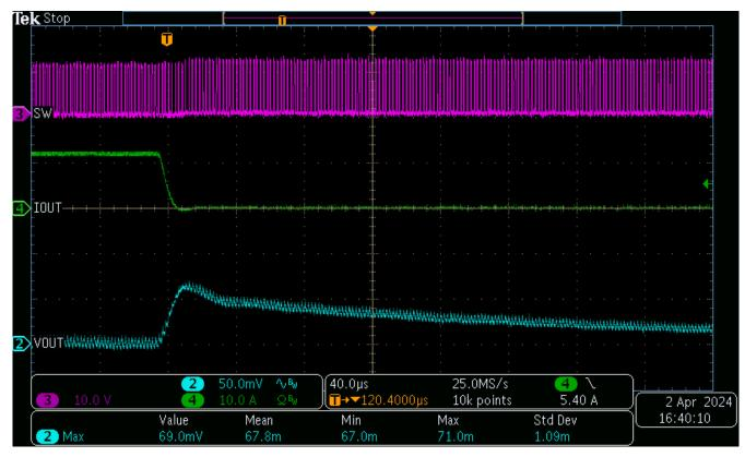
Figure 5-4. Transiant Response to Load Step 12A to 100mA at 8A/ $\!\mu s$
