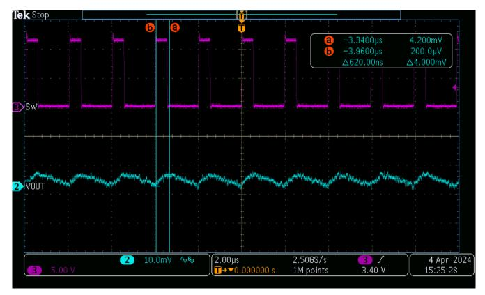
Figure 5-2. Output Voltage Ripple
