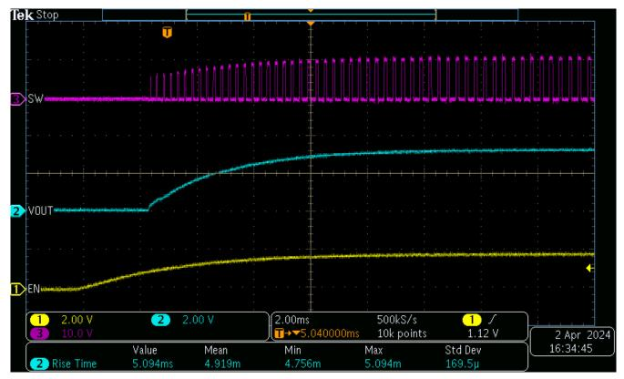
Figure 5-1. Soft Startup Into  $275m\Omega$  Load
