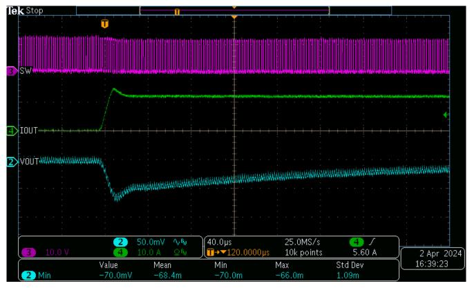
Figure 5-3. Transiant Response to Load Step 100mA to 12A at 8A/ $\!\mu s$
