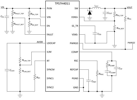
Figure 3-1. Simplified Schematic
