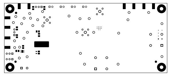
Figure 6-12. Bottom Solder Mask
