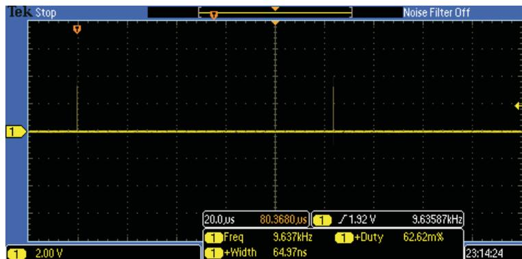
**Figure 1. Capture of glitch at PWM1 set to 0% duty cycle**
