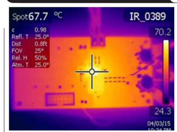
input and 1.2-V output at 20 A. Conditions for the TPS544B25 were a 12-V input and 0.95-V output at 20 A. The TPS40400 controller solution reached a maximum temperature of 47°C, while the TPS544B25 converter reached a maximum temperature of 67.7°C. These images show that spacing the MOSFETs away from the controller can enable better thermal performance and reduce the risk of causing failures or permanent damage to the board.
