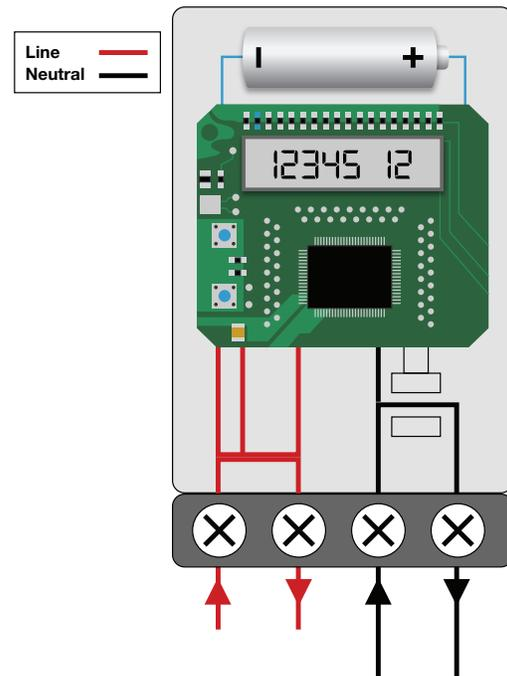
**Figure 1.** Example electricity meter configuration under normal operation.
