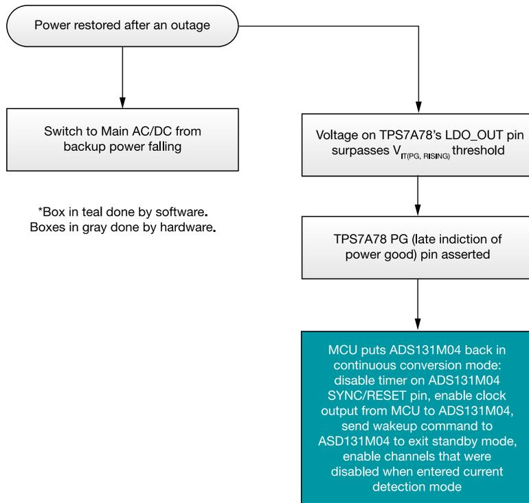
**Figure 6.** Sequence of events after power restoration.
