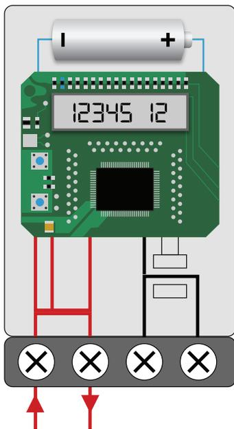
**Figure 2.** Example electricity meter configuration with neutral disconnected.
