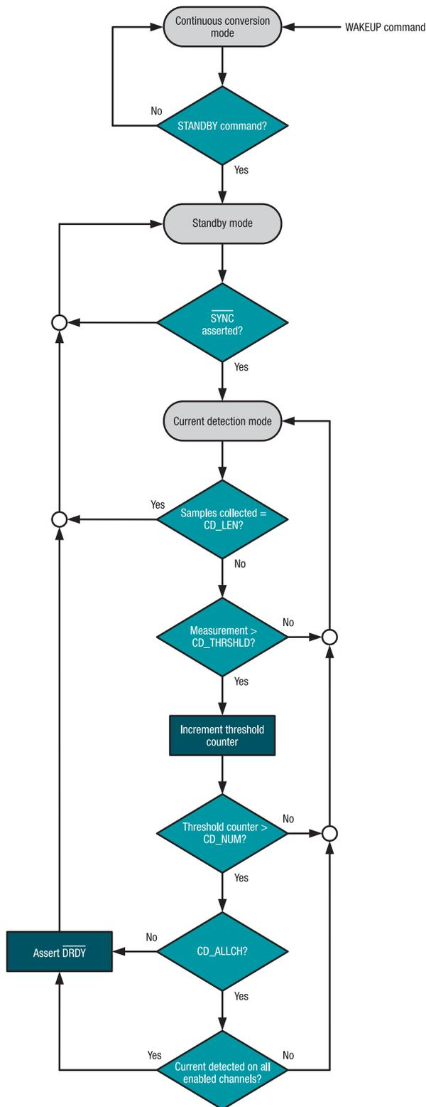
**Figure 3.** The current detection mode flow chart of the ADS131M04.
