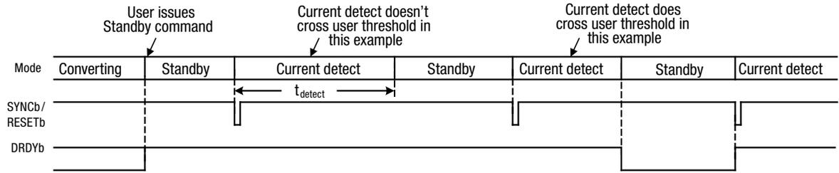
Figure 4. ADS131M04 current detection mode examples.
