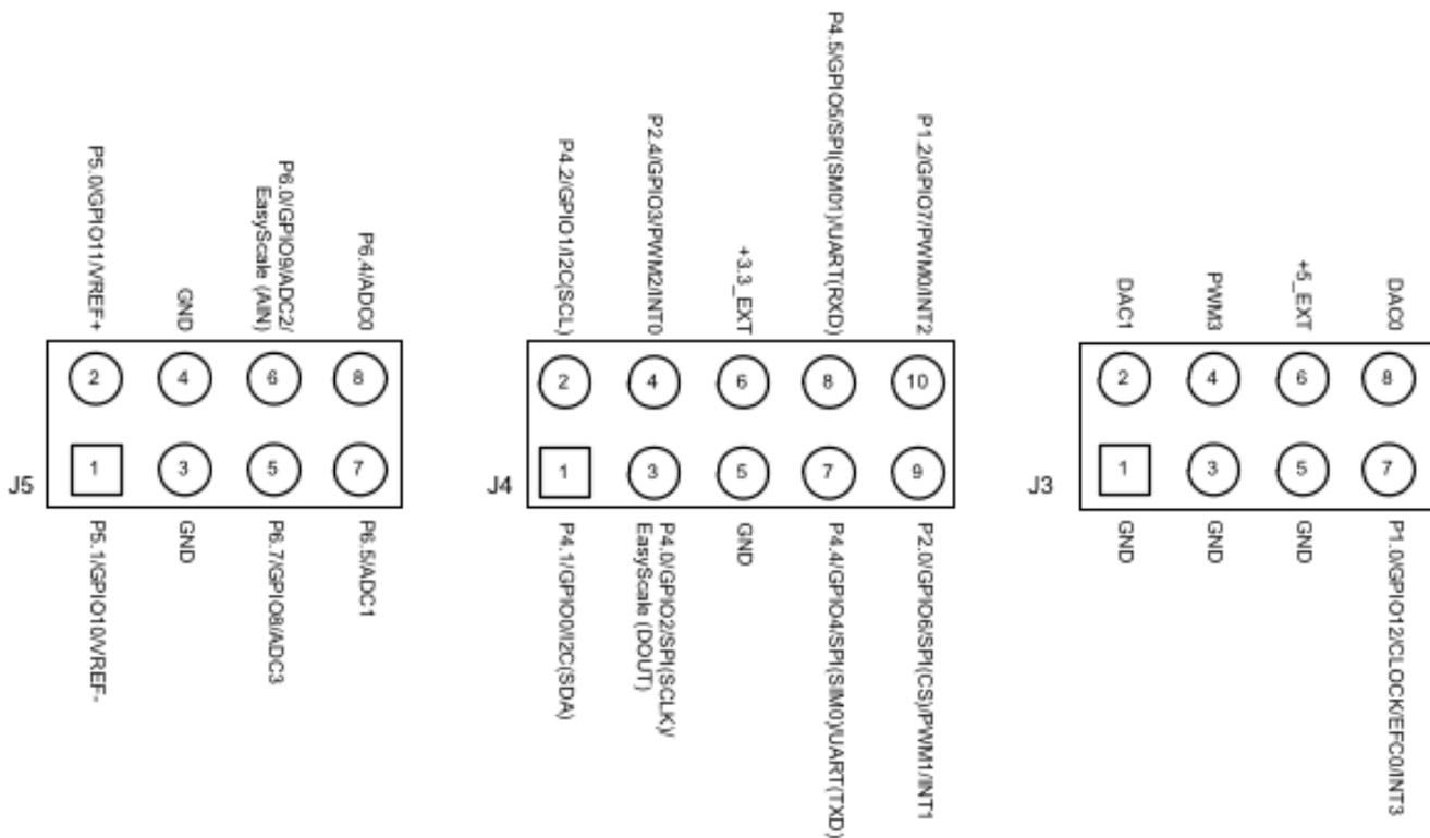
**Figure 16. USB2ANY Board Connector Pinout Diagram**
