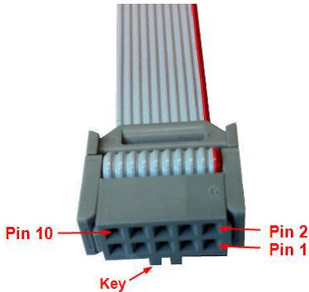
Figure 15. 10-pin Cable Pinout
