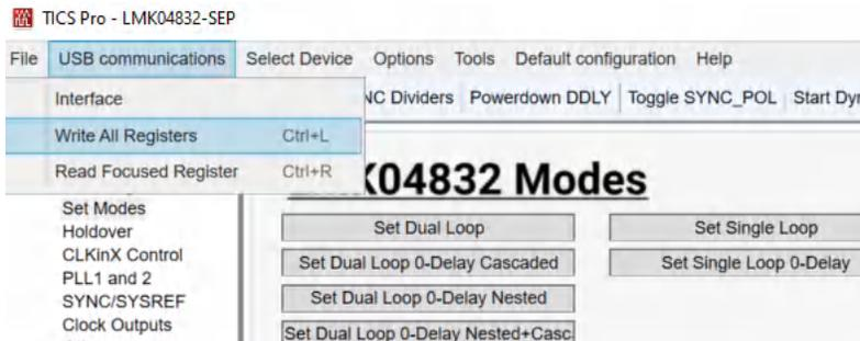
Figure 5-2. Loading the Device
