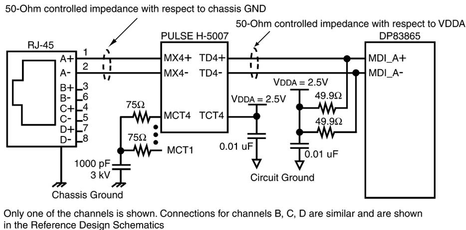
**Figure 8. Twisted Pair/Magnetics Interface (Channel A)**
