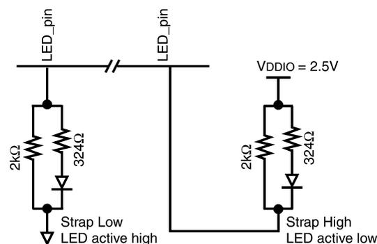
Figure 11. LED/Strapping Option examples
