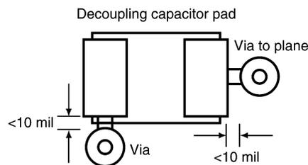
**Figure 2. Place Via Close to Pad**
