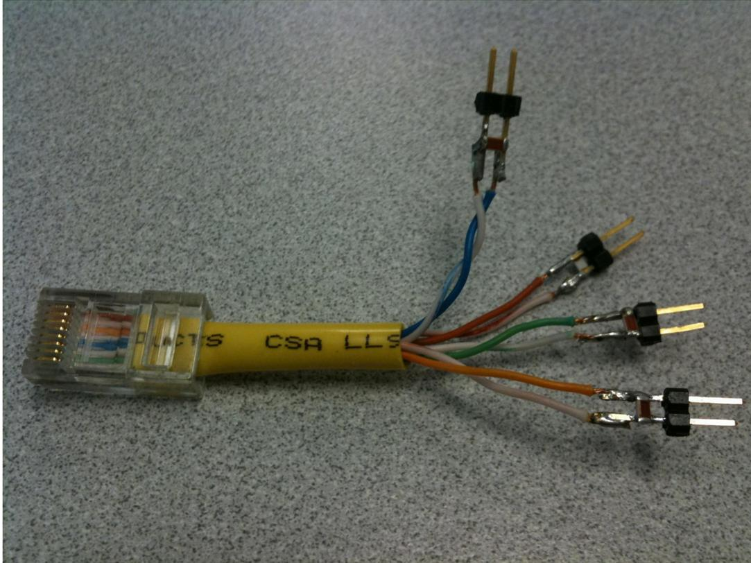
**Figure 3-2. 100 Ω Terminated Cable for MDI Signal Measurement**
