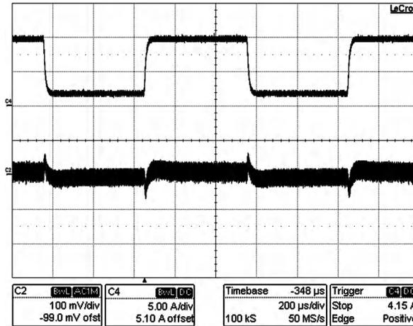
**Conditions:** Input Voltage = 48V DC Output Current = 2A to 10A **Traces:** Top Trace: Load Current, Amp/div = 5A Bottom Trace: Output Voltage Volt/div = 100mV, AC coupled Bandwidth Limit = 20MHz Horizontal Resolution = 0.2ms/div
