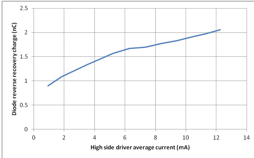
**Figure 7. Diode Reverse Recovery Change vs. High-Side Driver Average Current**
