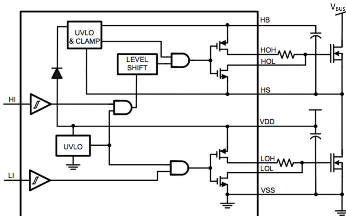
Figure 1. Block Diagram with External GaN FETs
