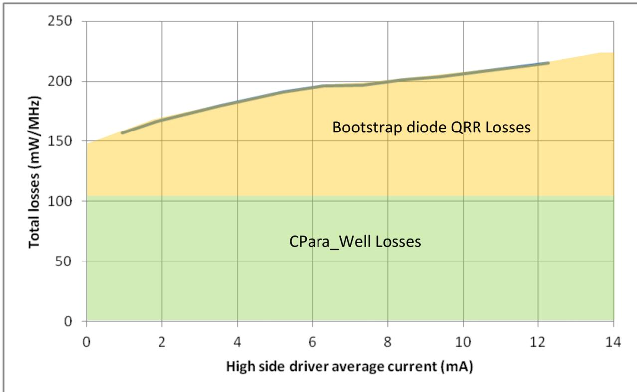
**Figure 5. Gate Driver Related System Losses per Mhz vs. Gate Drive Current at 50 V<sub>BUS</sub>.**
