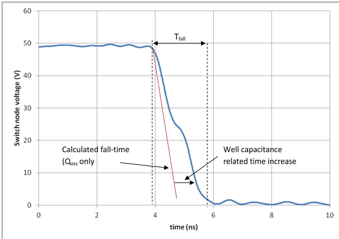
**Figure 6. Switching Voltage vs. Time (ns)**
