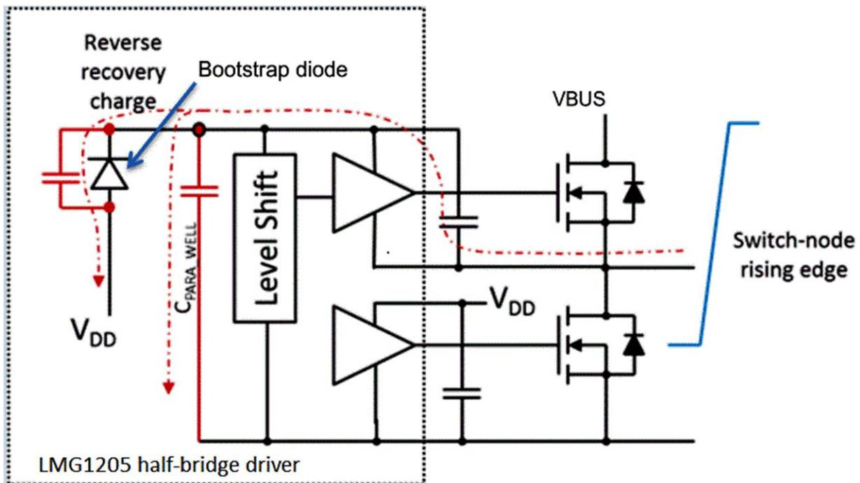
Figure 4. Partial Driver and Bridge Circuit
