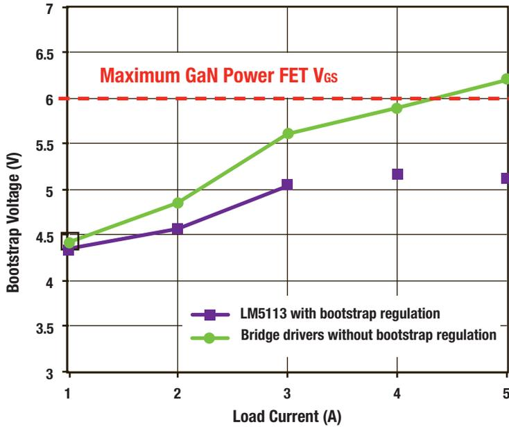
LM5113 bootstrap voltage regulation, synchronous buck converter evaluation board. input 48V; output 10V; switching frequency at 800 KHz.
