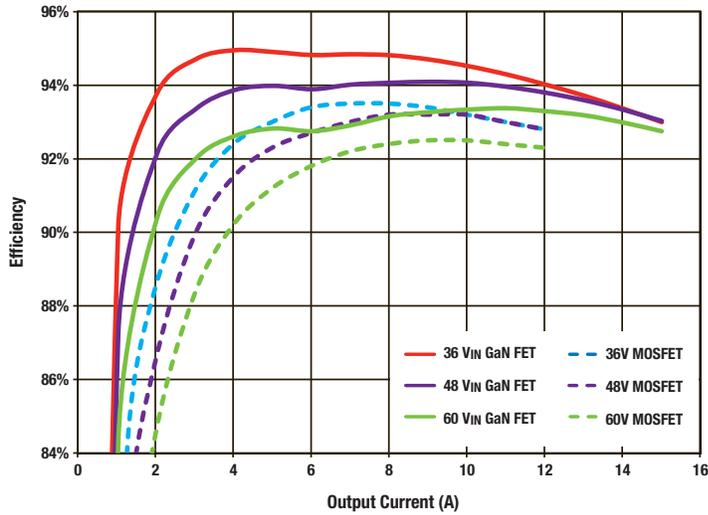
GaN FET efficiency vs traditional MOSFET. Input 36 to 75V; regulated output 12V; switching frequency at 333 KHz GaN FET, 250 KHz MOSFET.
