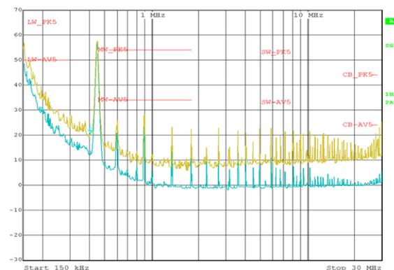
Figure 8. Conducted EMI Test Result 150kHz to 30MHz
