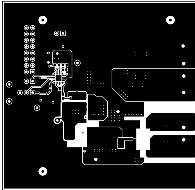
Figure 13. Top Copper (Top View)
