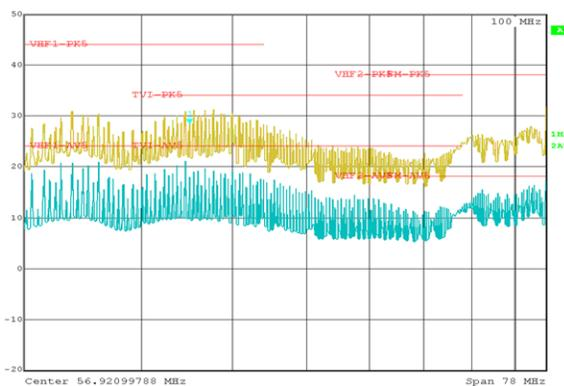
Figure 9. Conducted EMI Test Result 30MHz to 108MHz
