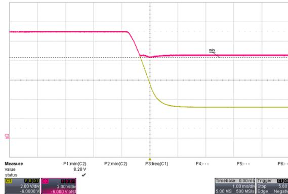
Figure 5. Cold-Cranking Using Cranking Simulator(C1:V<sub>SUPPLY</sub>, C2: V<sub>LOAD</sub>)
