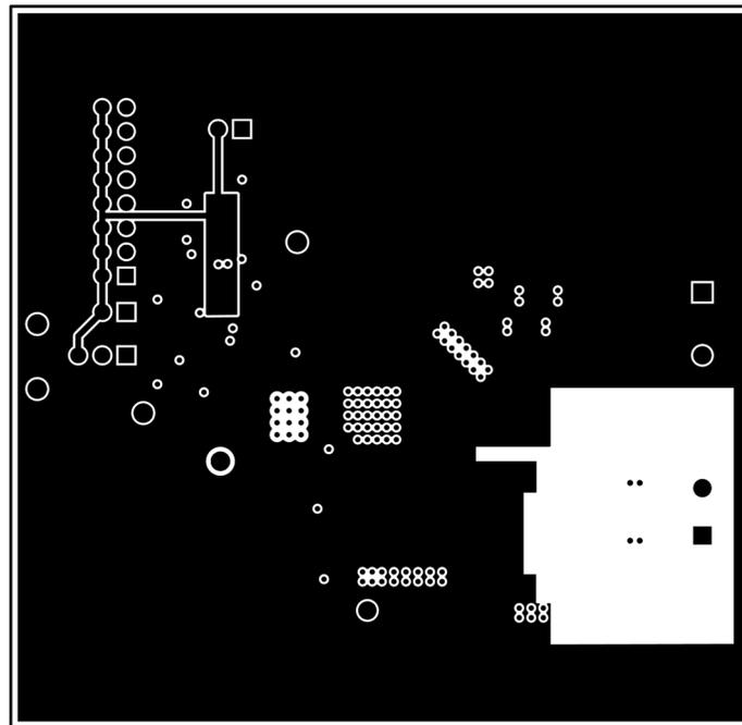
Figure 14. Mid1 Copper (X-Ray View)
