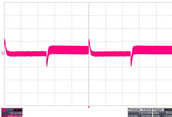
Figure 7. Load Transient(C2:V<sub>LOAD</sub> AC-coupled)
