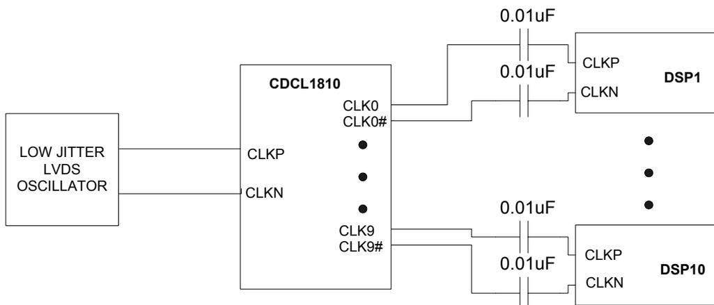
These buffers have not been tested but are examples of buffers that meet the specification requirements for all of the DSP differential clock inputs.
