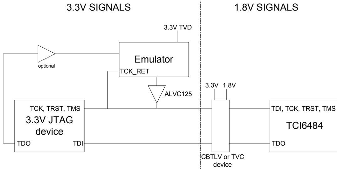
If the trace signals are supported, they may need to have voltage translation as well. Due to the speed of that interface, it is recommended that these signals be connected directly to the emulation header.
