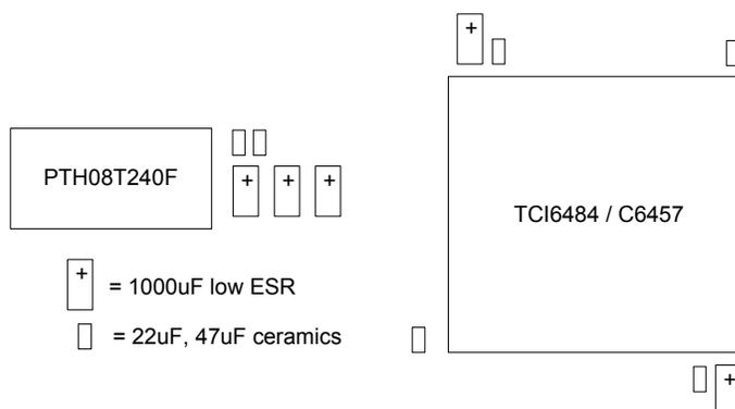
Each bulk capacitor should have reduced trace lengths less than 10 mils and contain multiple vias to tie the pad to the respective power plane. It is recommended that all bulk capacitors be low-ESR types. The acceptability of each output capacitor should be based on the following criteria:
