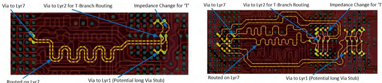
**Figure 3-8. Example LPDDR4 Clock and CA Routing**
