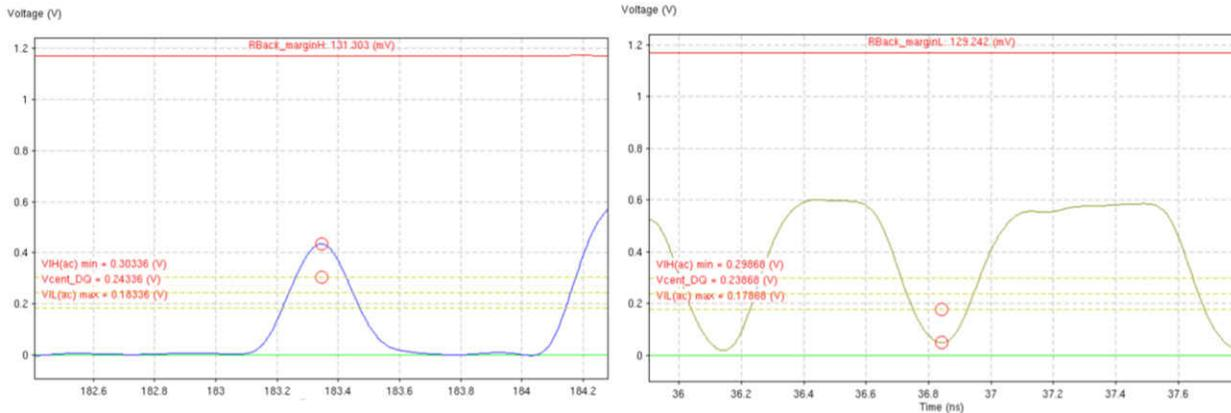
Figure 3-3. Example of Ring-back Margin Waveforms (High/Low)
