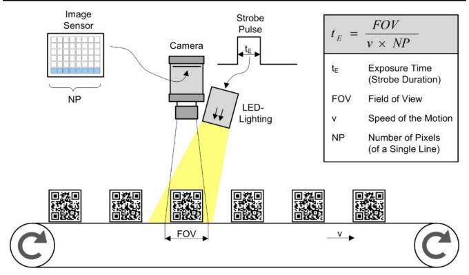
Figure 1. Typical Setup for a Machine Vision System: Short Strobe Pulses Freeze the Motion of the Objects on the Conveyor Belt
