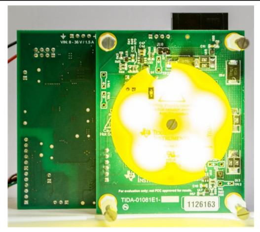
Figure 2. LED-lighting Control Reference Design for Machine Vision with the LEDs Switched on
