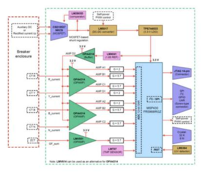
Figure 1. Signal Processing Subsystem and Current Input-Based Self Power for Breaker Applications
