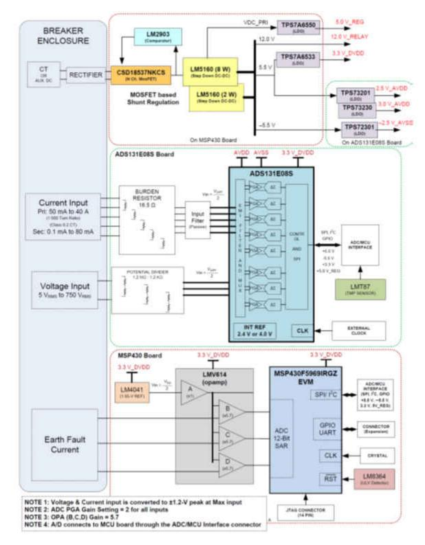
Figure 2. Analog Front End for ACB Block Diagram
