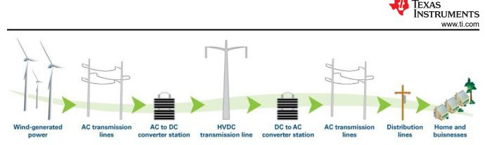
Figure 1. Transmission Process(image Courtesy of Duke American Transmission Lines)
