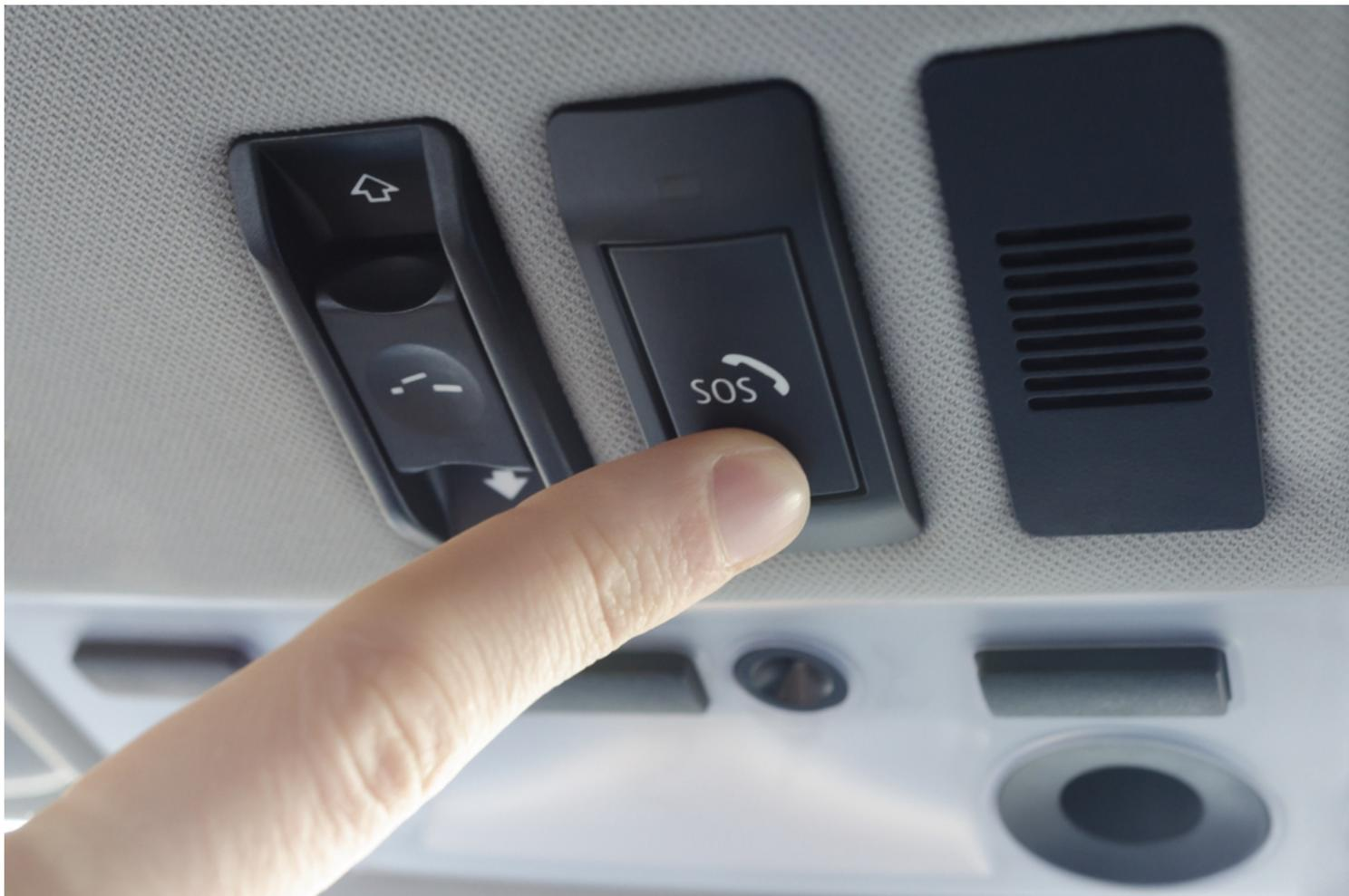
Many government regulators have considered requiring emergency call (eCall) systems in automobiles. An eCall system will automatically contact emergency responders in the event of a serious road accident, send GPS coordinates to local emergency services, and wirelessly send airbag-deployment and impact-sensor information.
