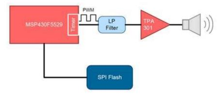
The example code framework can be made to cycle through several stored audio samples when the appropriate LaunchPad button is pressed, this framework can be easily modified or alternatively the core functions may be incorporated into almost any MSP430 MCU application. By using simple "#define" statements, the user can select from several different MSP430 MCU LaunchPad kits and can also configure playback for various pre-defined frequencies.
