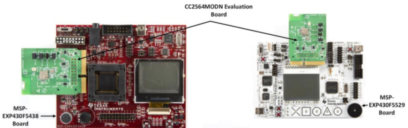
Figure 2. Hardware Setup
