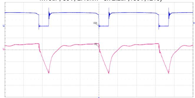
48Vin, 12Vout, 5A Load, 1.274V (2.65%) (1x68uF, 100V, 320mohm +1x10uF, 80V, 2.4ohm+ 3x 2.2uF,100V,1210)
