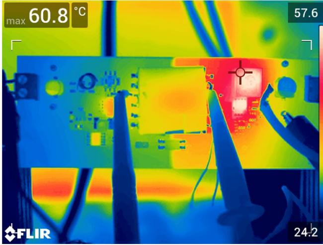
48Vin, 12V5A,  $T_{FET(SEC)}=60.8C$  Front view
