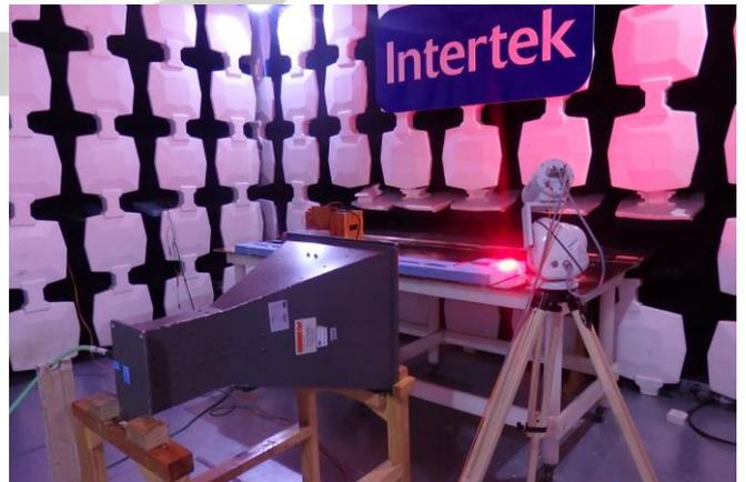
Picture for general setup (above 1GHz)
