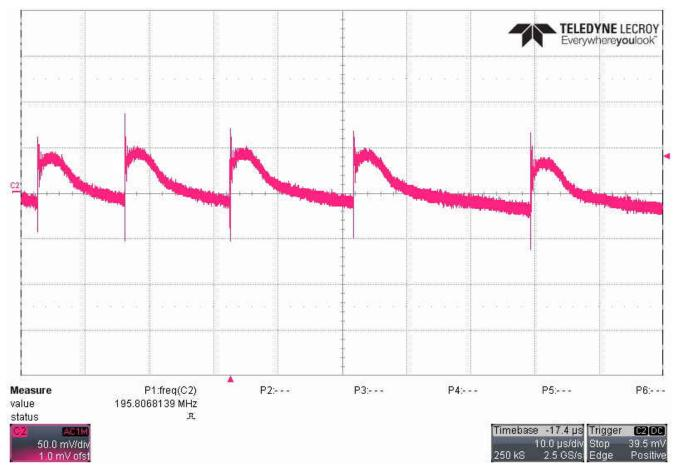
Figure 3-3. Output Voltage Ripple 1
