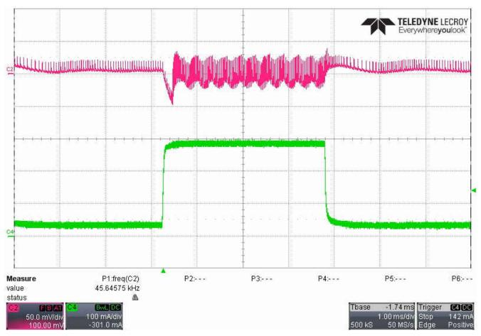
Figure 3-4. Load Transient
