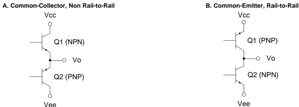
Figure 1. Simplified Output Stages
