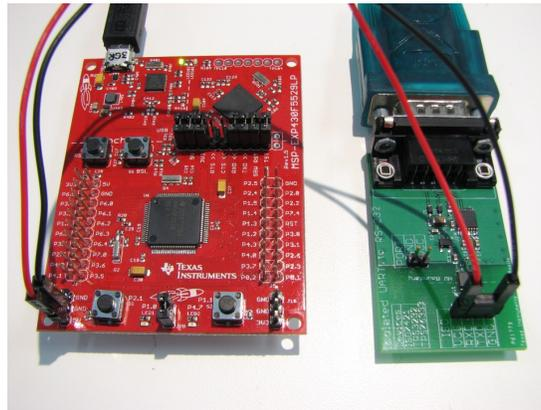
**Figure 2. Hardware Loopback**
