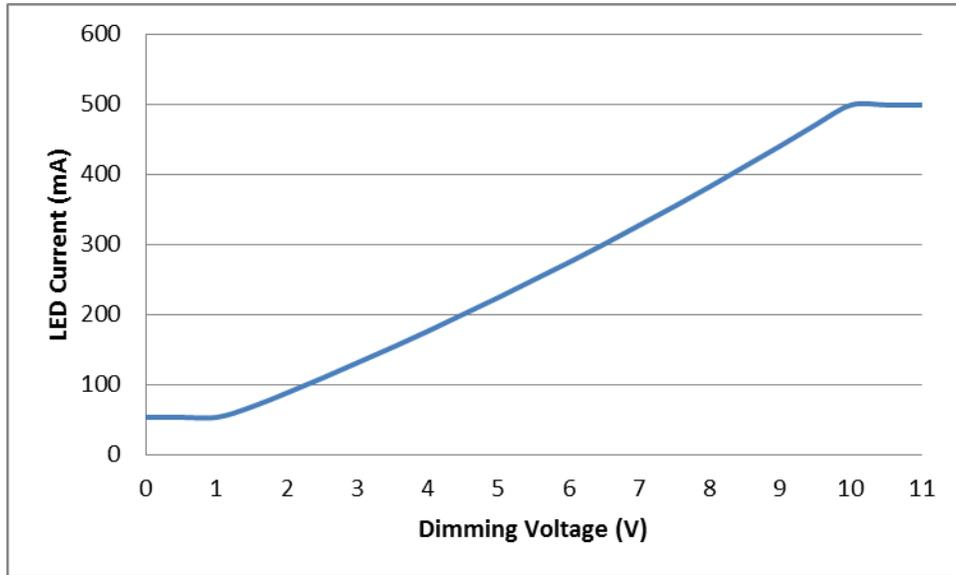
Figure 7: LED Current vs. Dimming Voltage
