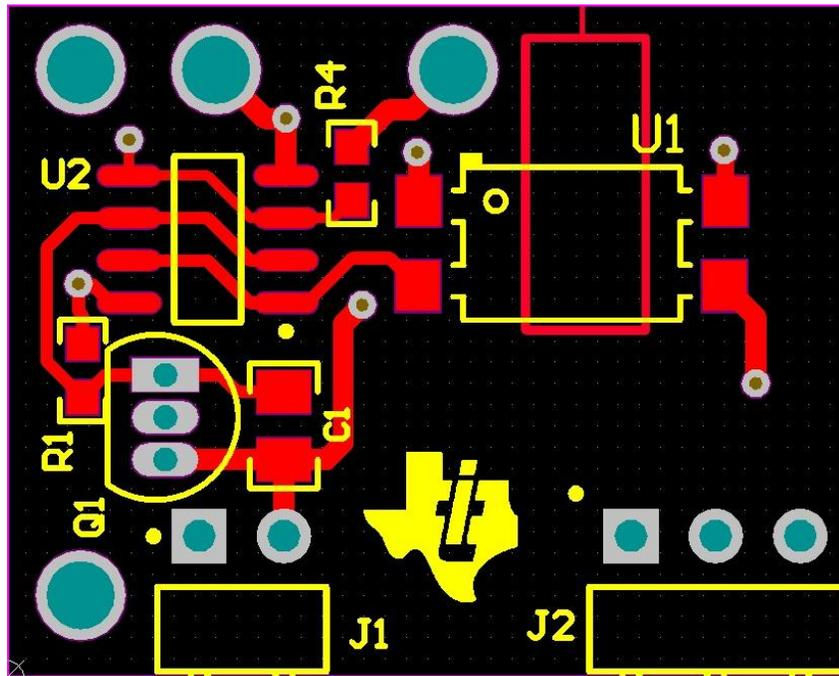
Figure 18: Top Layer and Top Overlay Daughter Board (Top view)
