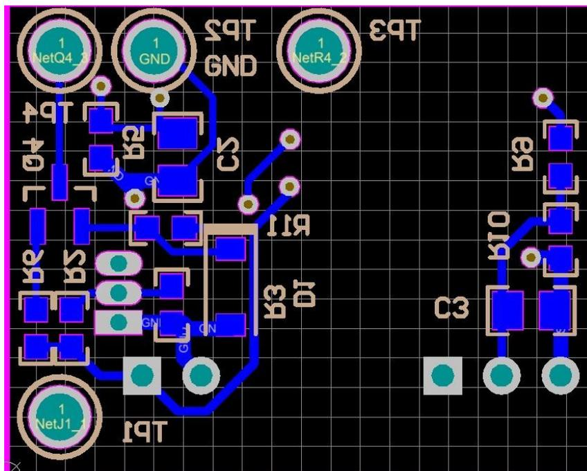
Figure 19: Bottom Layer and Bottom Overlay Daughter Board (Bottom view)
