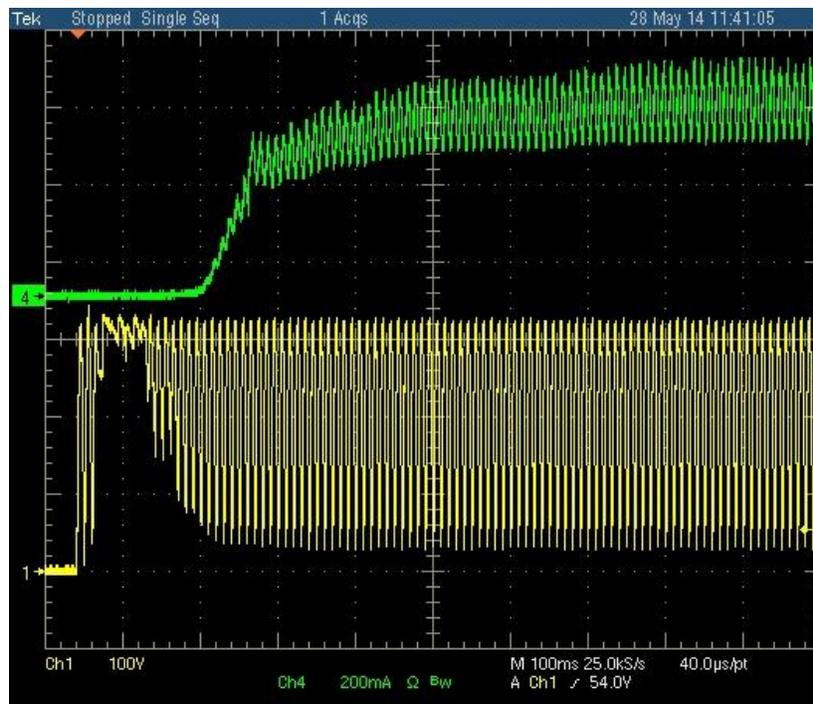
**Figure 9: Start Up Waveforms at 230Vac 50Hz Ch1: Rectified AC Input Ch4: LED current**
