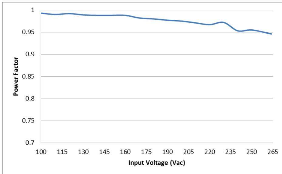
**Figure 6: Power Factor 50Hz**
