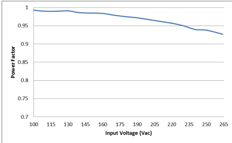
**Figure 5: Power Factor 60Hz**
