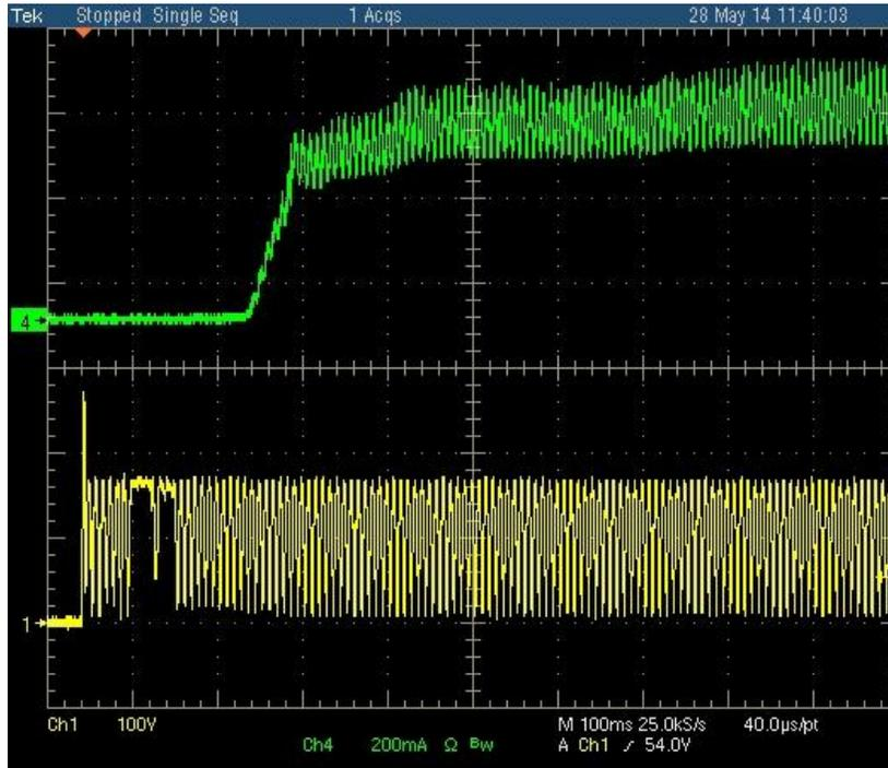
**Figure 8: Start Up Waveforms at 120Vac 60Hz Ch1: Rectified AC Input Ch4: LED current**
