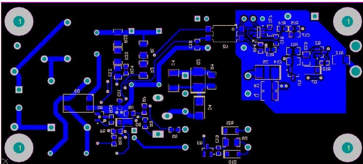
Figure 17: Bottom Layer and Bottom Overlay Main Board (Bottom view)
