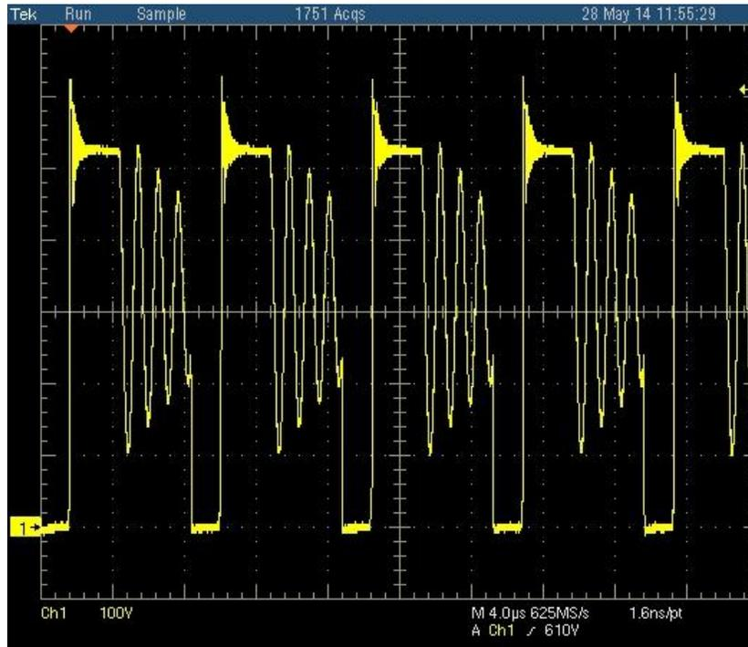
Figure 13: Switch Node at 230V 50Hz Ch1: MOSFET Q6 Drain
