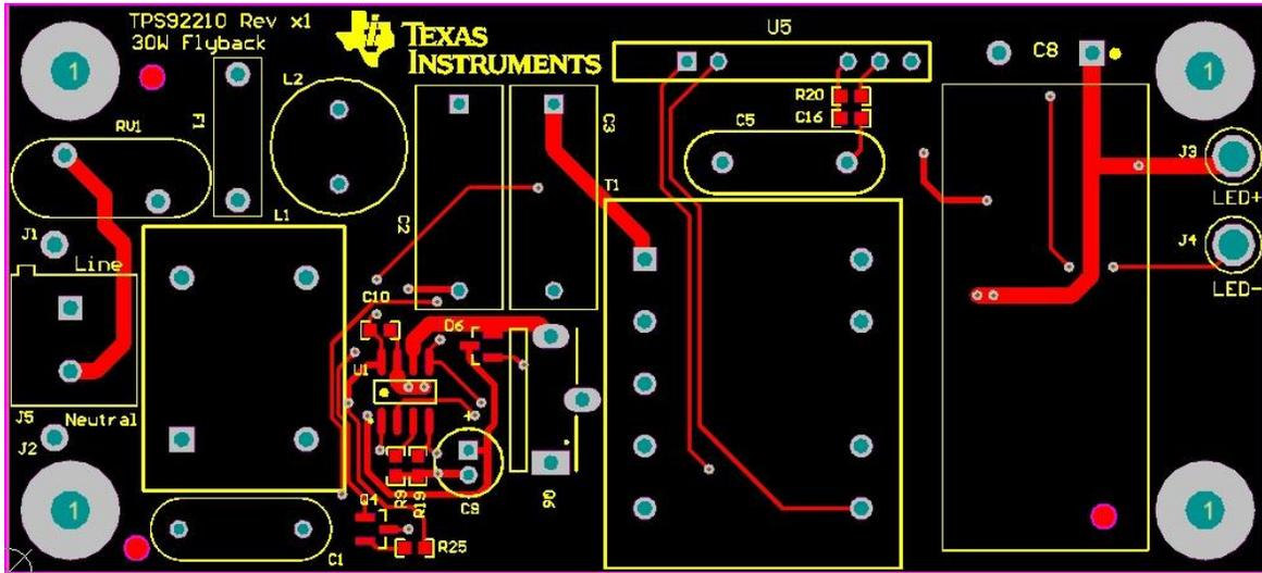
Figure 16: Top Layer and Top Overlay Main Board (Top view)
