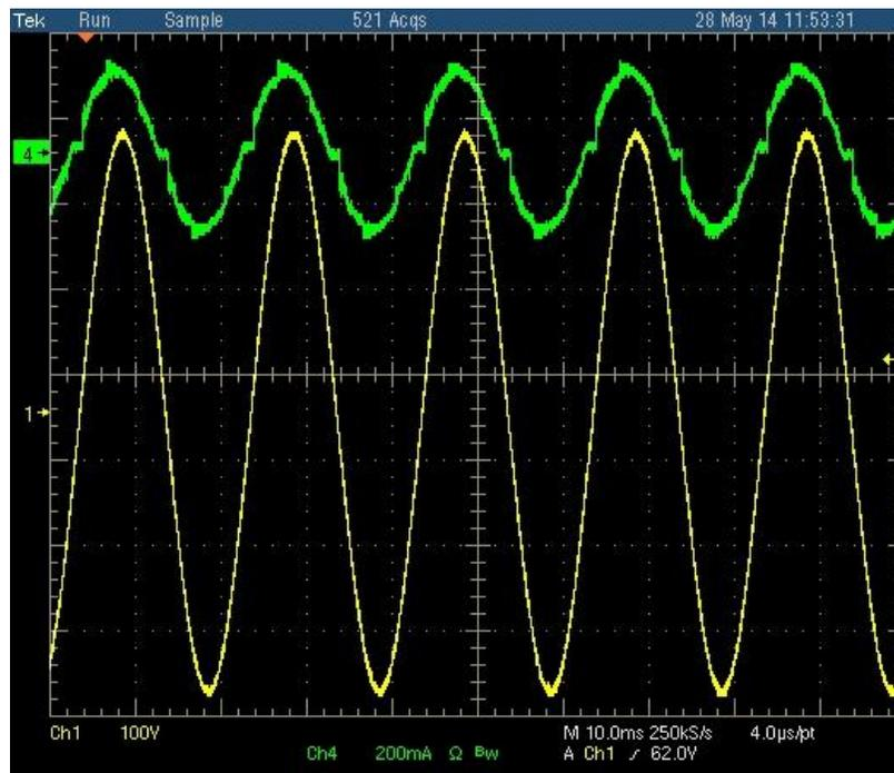
**Figure 11: Input Current at 230V 50Hz Ch1: Input Voltage Ch4: Input Current**
