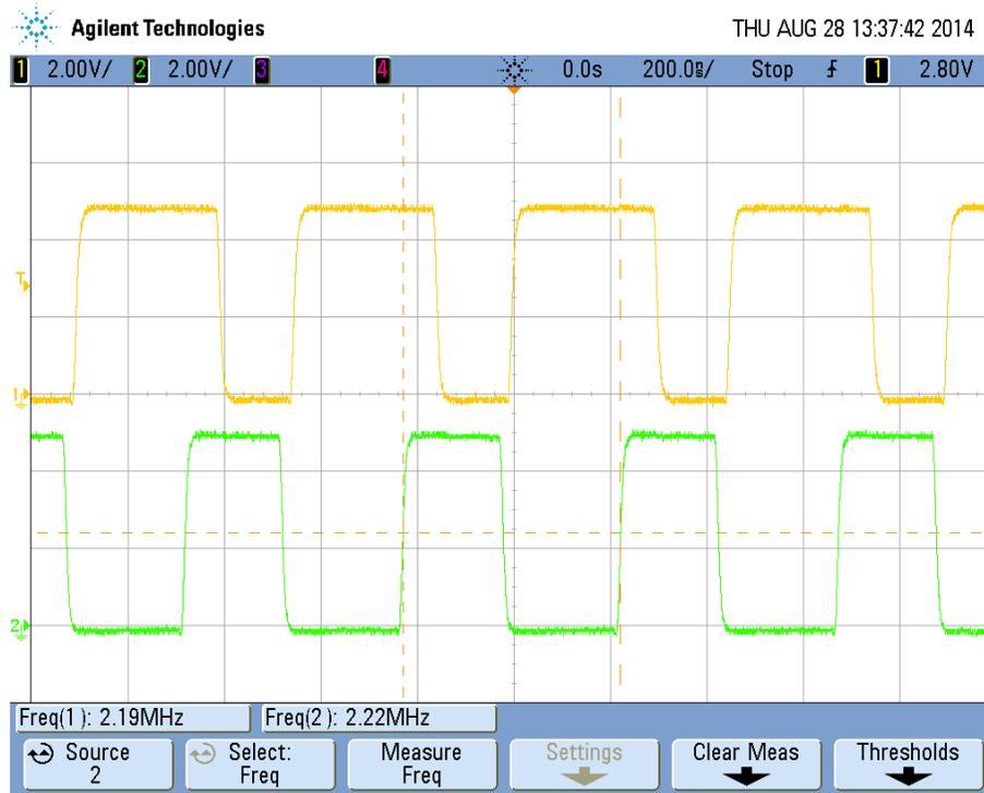
Figure 13 Switch Node Waveforms for the 2.8V and 1.8V Buck at Full Load
