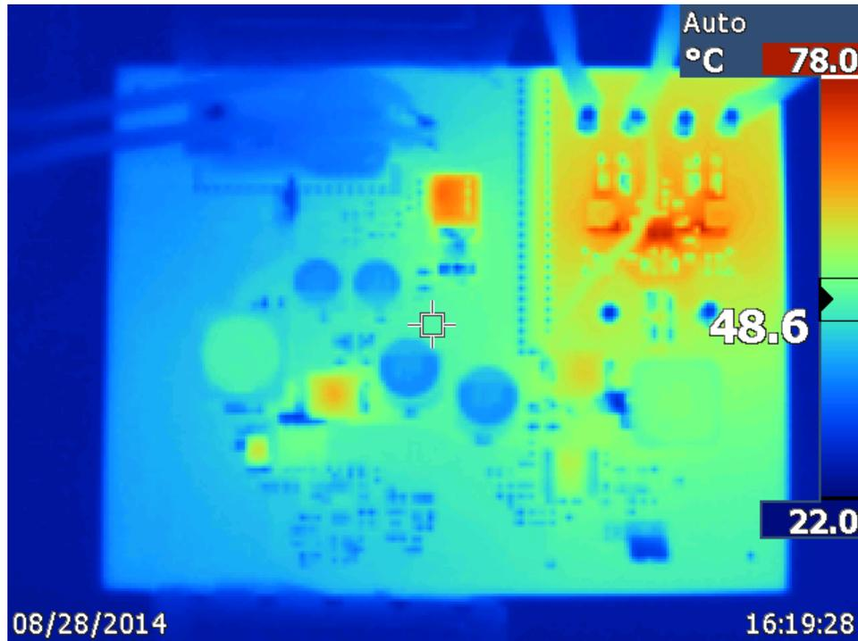
Figure 3 Board Thermal Image at 4.5V input
