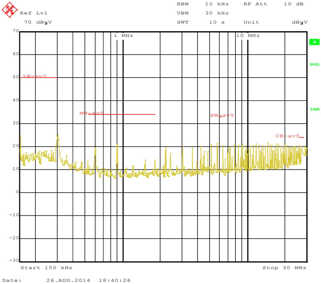
Figure 16 Peak detect, 150kHz – 30MHz
