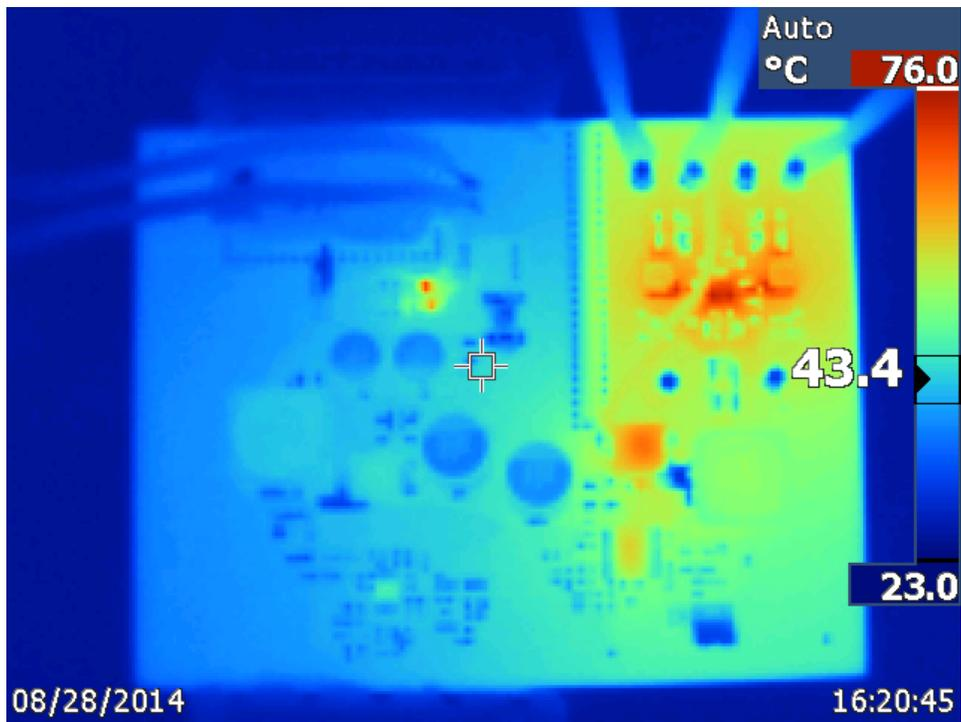
Figure 5 Board Thermal Image at 38V input
