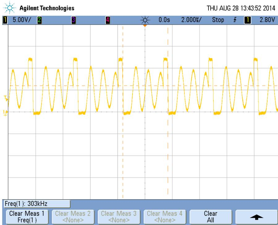
Figure 12 Switching Waveform for the 5V Buck at 12Vin and No Load
