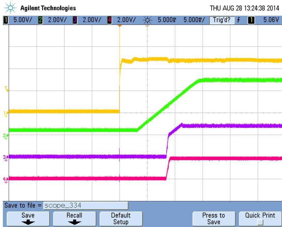
Figure 19 Start Up into Full Load at 12Vin
