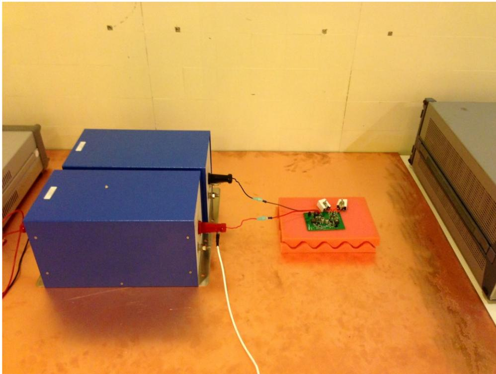
**Figure 15 Conducted EMI Test Setup**
