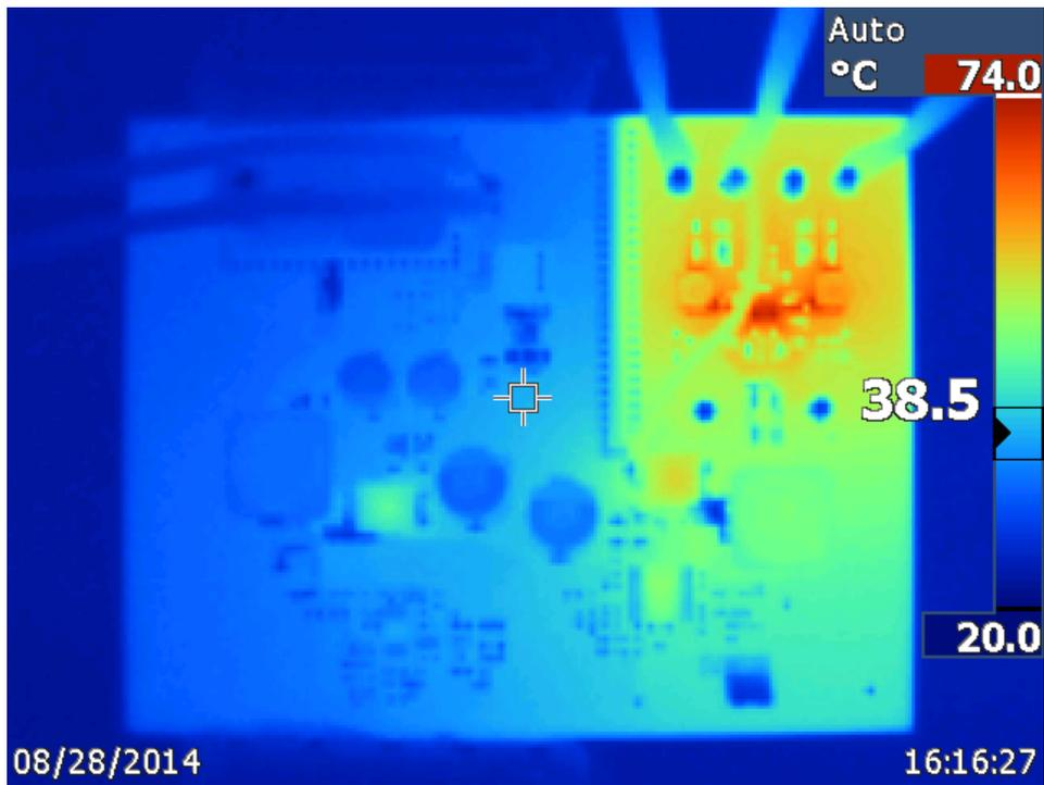
Figure 4 Board Thermal Image at 12V input
