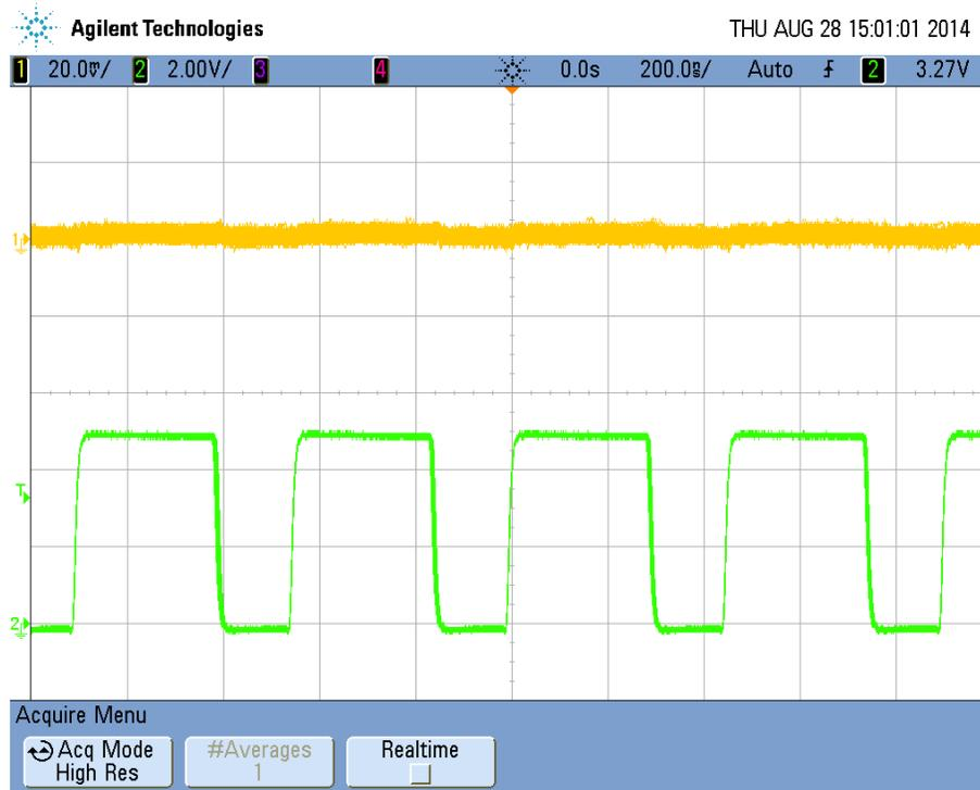
Figure 26 2.8V Output Ripple at 2A Load
