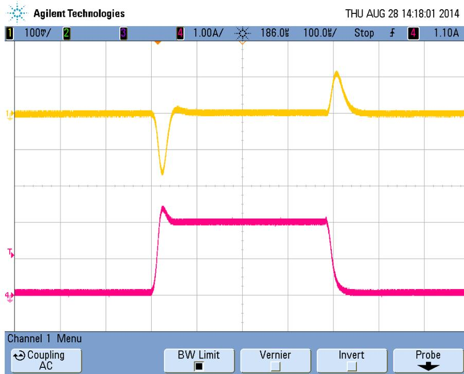
Figure 23 1.8V Output Buck Regulator Load Transient
