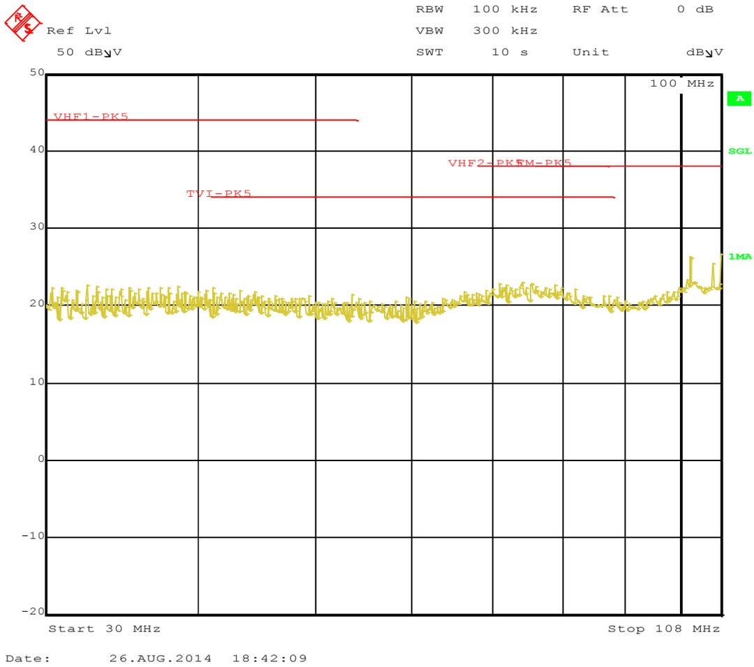
Figure 17 Peak detect, 30MHz – 108MHz
