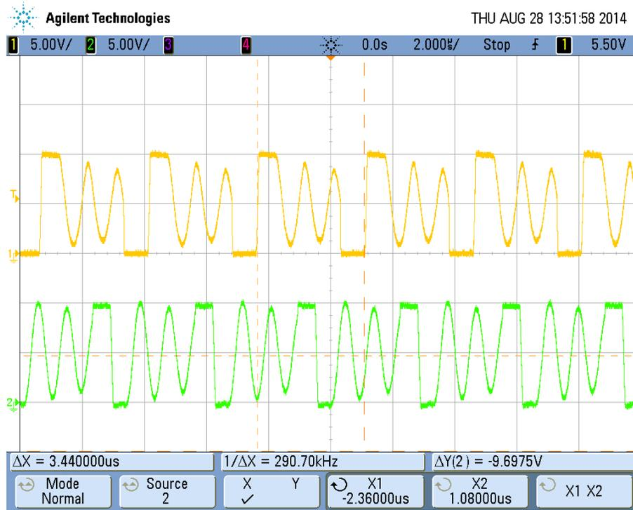
**Figure 10 Switching Waveforms for the Pre-boost and the 5V Buck at 4.5Vin and No Load**
