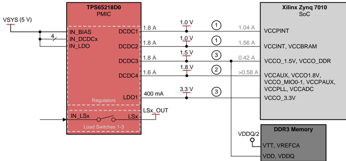
Table 2 lists the voltage settings required for the TPS65218D0 to power the Xilinx Zynq 7010 properly.
