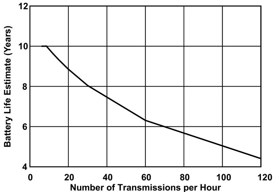
**Figure 17. Battery Life Estimation versus Number of Transmissions per Hour for TIDA-00758**
