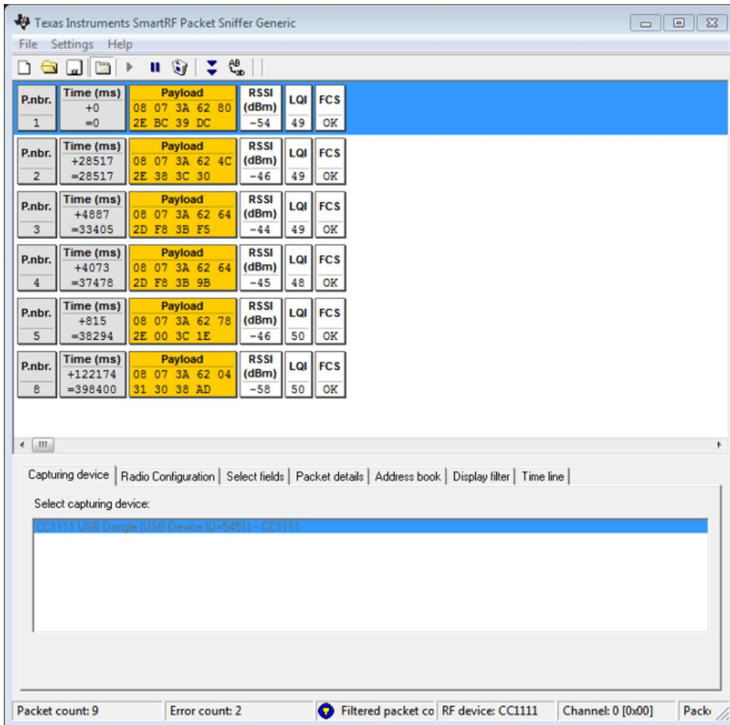
Figure 15. Filtered Radio Data
