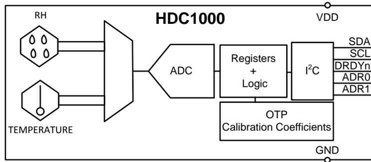
**Figure 6. HDC1000 Functional Block Diagram**
