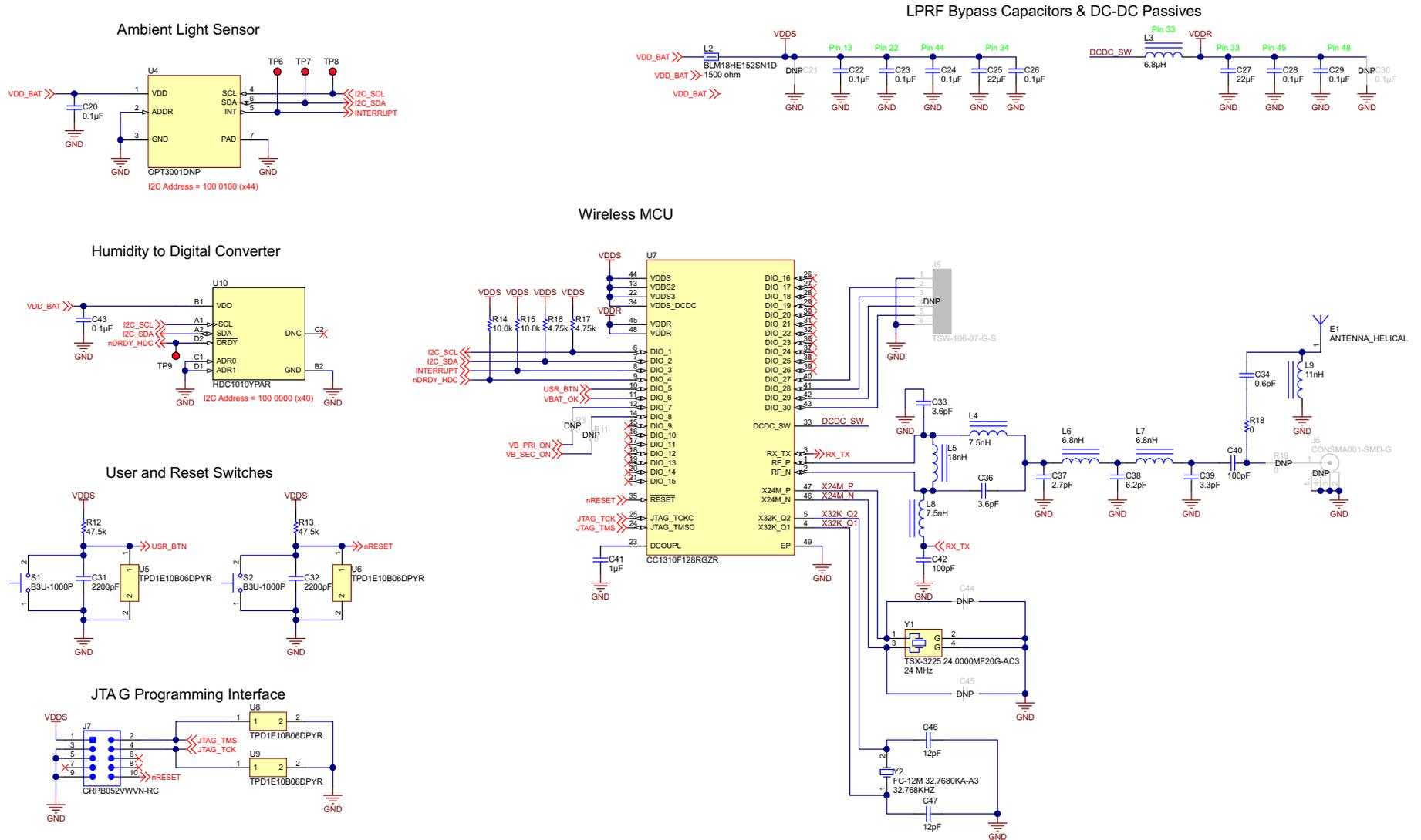
Figure 20. Bluetooth® and Light Sensing Schematic
