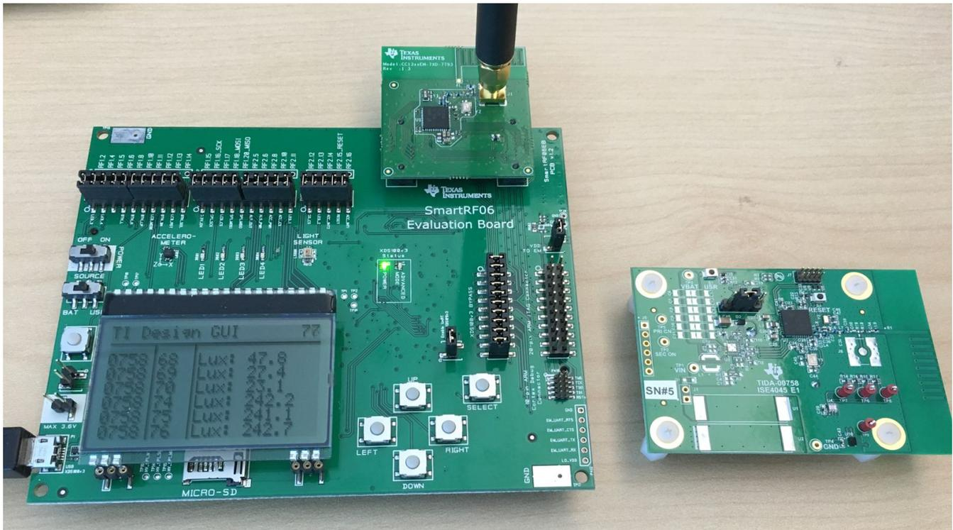
**Figure 11. Sniffer Application Firmware Running on the SmartRF06 EVM With TIDA-00758 and TIDA-00488 Reference Designs**
