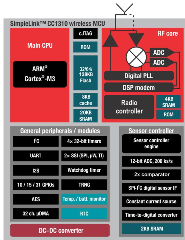
**Figure 3. CC1310 Functional Block Diagram**
