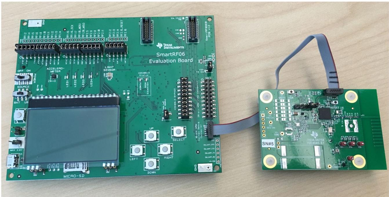
**Figure 10. Connection of SmartRF06 EVM and TI Designs Hardware for Programming and Debugging**
