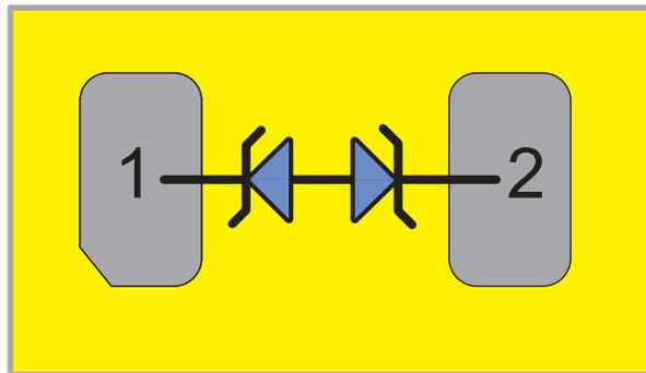
**Figure 7. TPD1E10B06 Functional Block Diagram**
