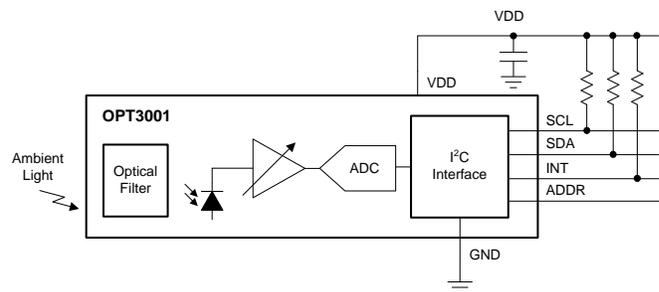
Figure 5. OPT3001 Functional Block Diagram
