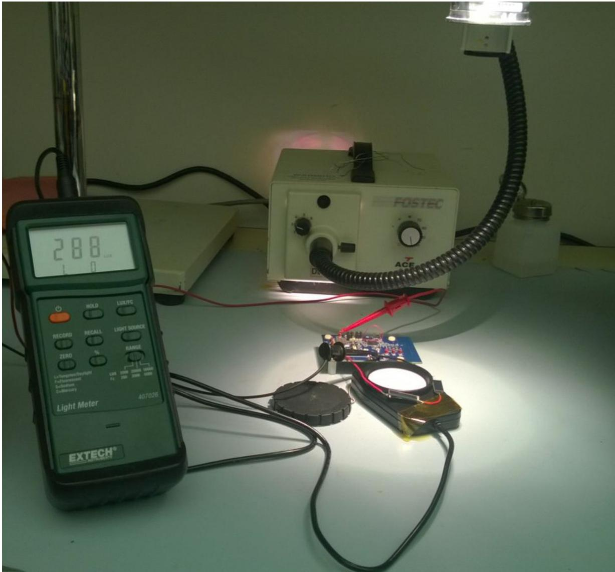
**Figure 18. Light Measurement Setup for Verifying the OPT3001 Trip Points**
