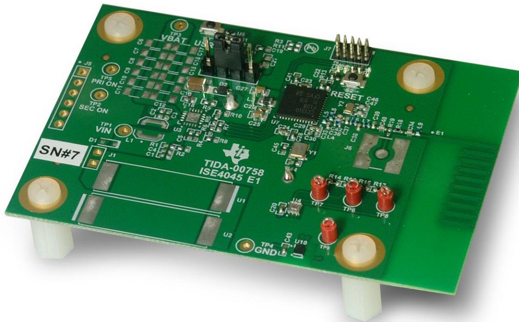
**Figure 9. Interrupt-Based Ambient Light and Environment Sensor Node for Sub-1GHz Networks Reference Design Hardware**
