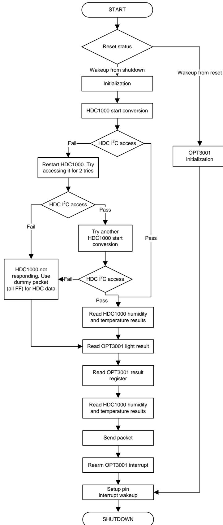
Figure 8. Firmware Flowchart
