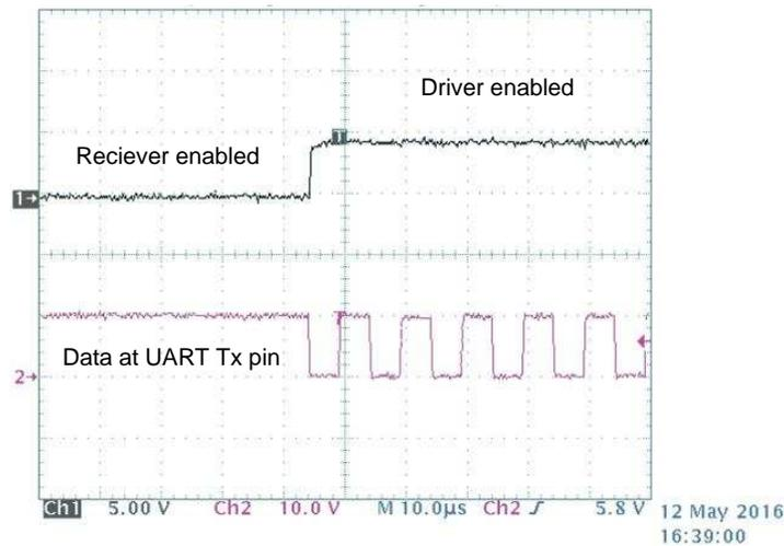
Figure 8. Enable Signal for 200 kbps
