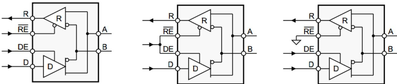
**Figure 1. Half-Duplex Transceiver Configuration**
