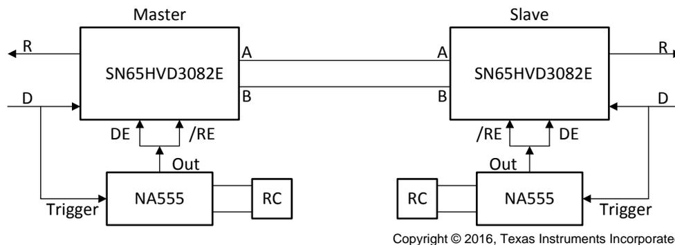
**Figure 2. Automatic-Direction Control RS485-Block Diagram**
