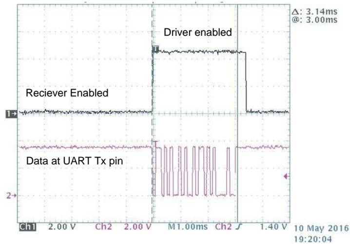
Figure 5. Plot of Data Transmission and Direction Control Signal
