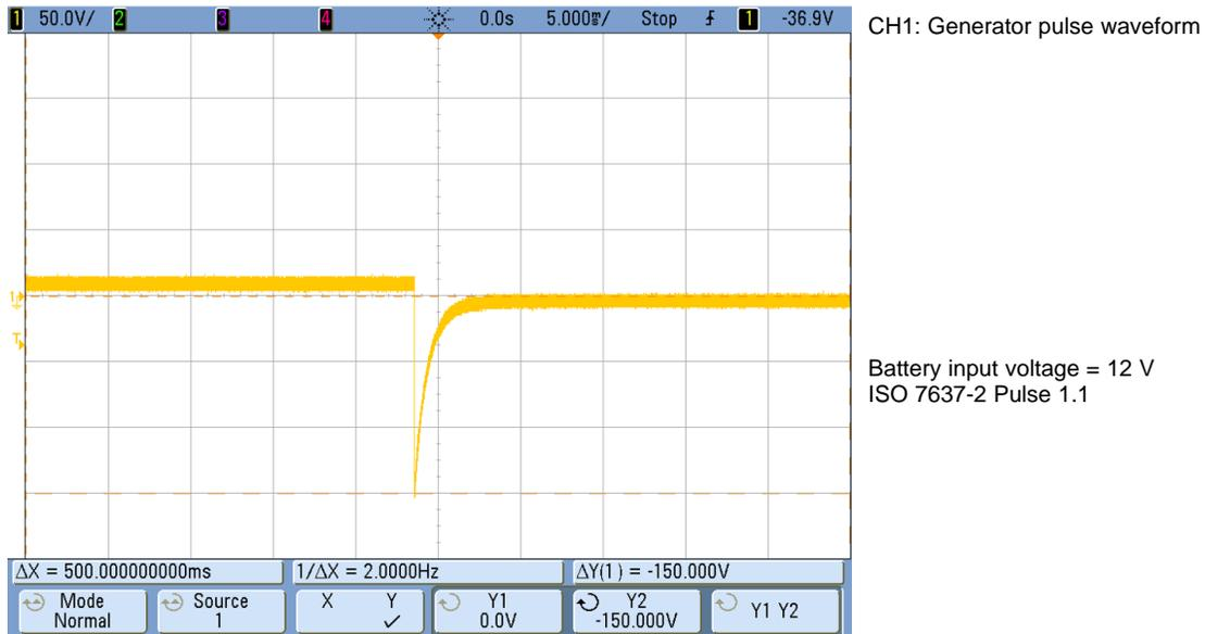
Figure 28. ISO 7637-2 Generator Pulse 1.1 at 12 V
