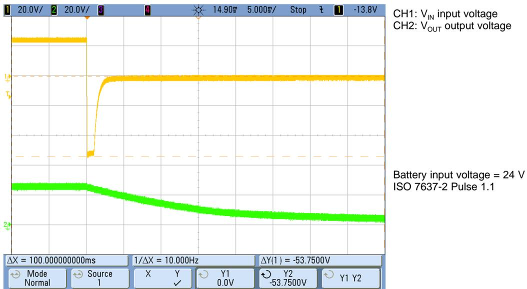
Figure 39. TIDA-00992 Pulse 1.1 at 24-V Behavior
