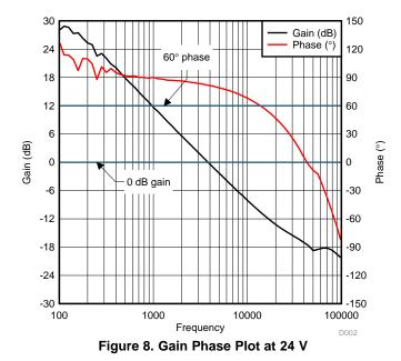
A margin of greater than 60 degrees satisfies the requirement for stable operation. This margin provides enough guardband for aging, temperature variation, and component variations. If the amount of guardband is not needed, then increase the gain up to 6 dB for a faster transient response.
