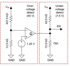
Figure 15. Principle Circuit for Disabling LM5001 at  $V_{IN} > 45$  V and  $V_{IN} < 7.5$  V
