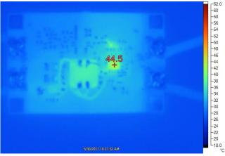
Figure 14. Thermal Image at V<sub>IN</sub> = 24 V
