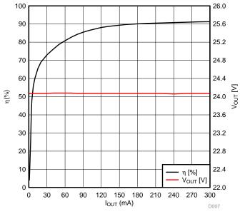
Figure 11. Efficiency at 24 V versus Load
