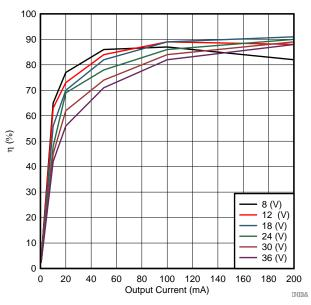
Figure 9. Efficiency versus Output Current
