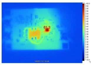
Figure 13. Thermal Image at  $V_{IN} = 8 V$
