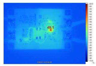
Figure 12. Thermal Image at V<sub>IN</sub> = 36 V
