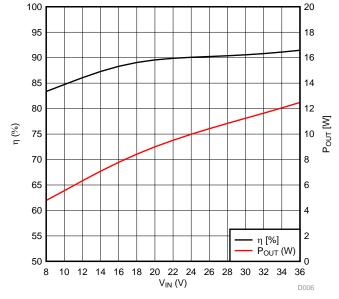
Figure 10. Maximum Power and Efficiency versus  $V_{\mbox{\tiny IN}}$
