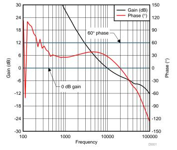
Figure 5. Gain Phase Plot Recorded by Frequency Response Analyzer From Venable Instruments
