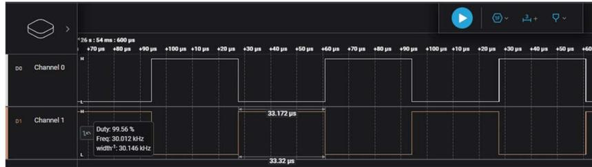
**Figure 4-14. Build Level 1: PWM Output Waveforms**
