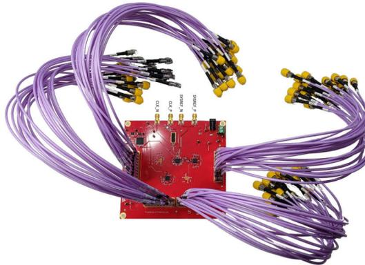
**Figure 3-2. Cascaded Clock Distribution Board with RF Cables**
