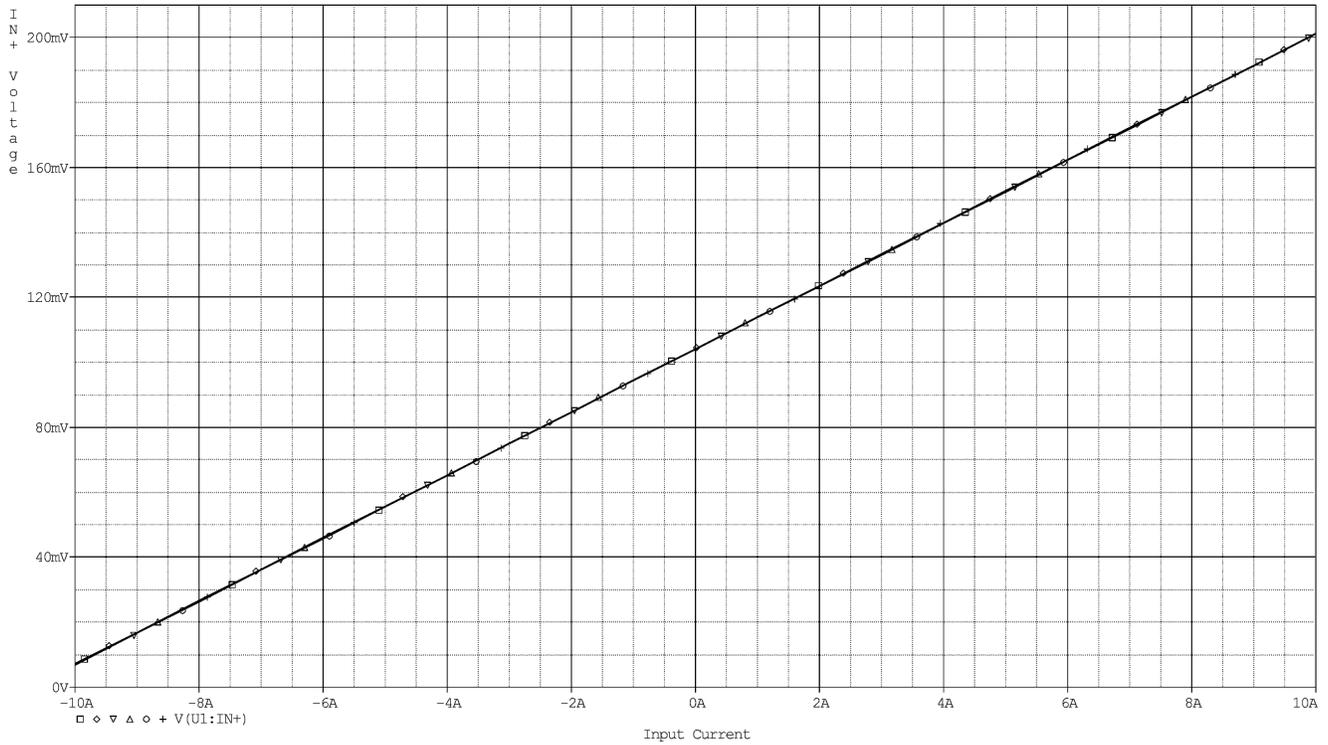
**IN+ Voltage vs Input Current**
