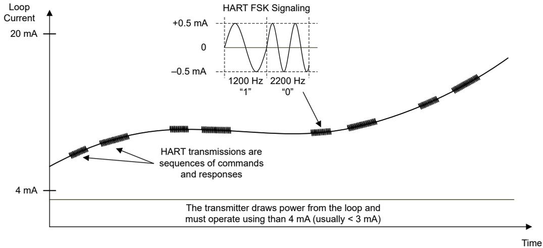
Figure 1-3. HART Transmissions on a 4-20 mA Loop
