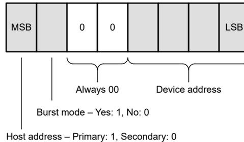
**Figure 1-11. HART Short Frame Address Byte**
