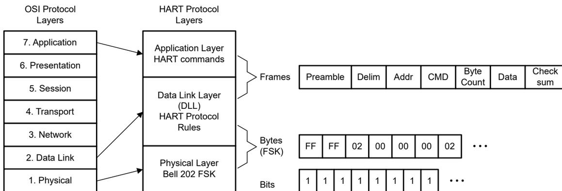
**Figure 2-1. HART Protocol Compared to the OSI Protocol Model**
