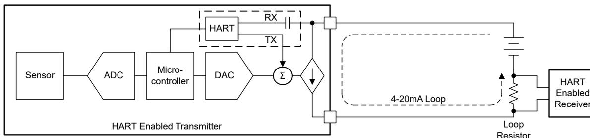
**Figure 1-2. Adding HART to the 4-20 mA Loop**
