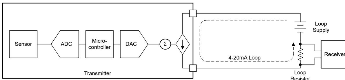
**Figure 1-1. A Remote Transmitter on a 4-20 mA Loop**
