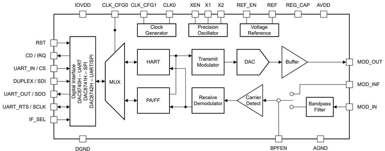
Figure 3-4. Block Diagram of the DAC874xH HART Modem
