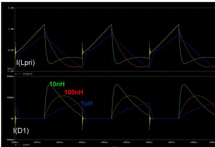
**Figure 3.** Recharge current wave shape is strongly impacted by leakage inductance. (Green = 10 nH, Red = 100 nH, Blue = 1  $\mu$ H)
