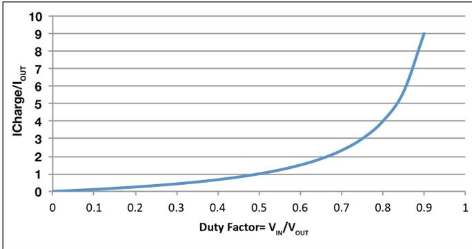
**Figure 2.** Capacitor C7 charge current is high for high duty factor or  $V_o$  near  $V_{in}$ .
