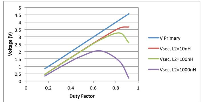
**Figure 4.** Leakage inductance is a killer on regulation.
