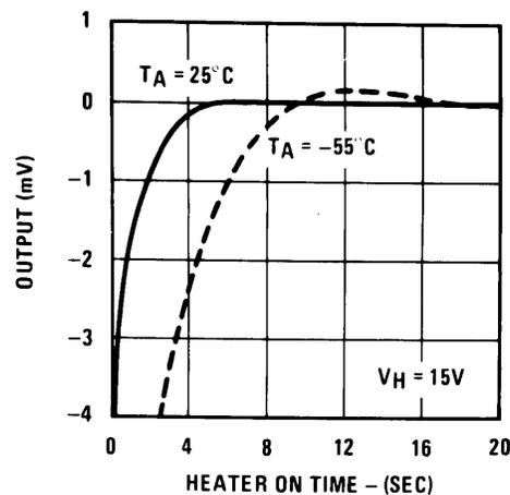
**Figure 7. Fast Warmup Time of the LM199**
