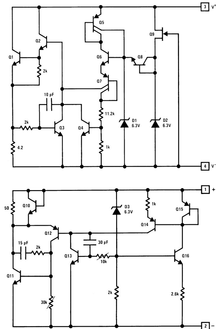
**Figure 3. Schematic Diagram of LM199 Precision Reference**
