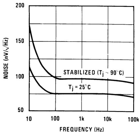
**Figure 5. Wideband Noise of the LM199 Reference**
