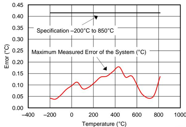
**Figure 47. Maximum Measured Error of the Complete System Across -200°C to 850°C**
