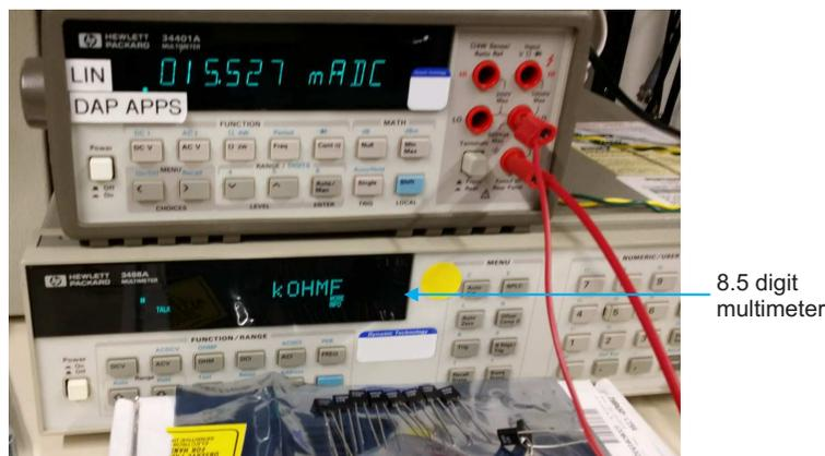
**Figure 40. Precision Resistors and an 8.5-digit Multimeter**
