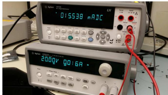
Figure 22. Power Supply and Multimeter Connected in Series
