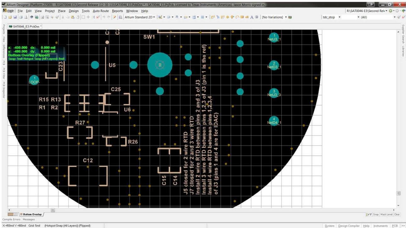
Figure 28. 2-Wire, 3-Wire, and 4-Wire RTD Support Shown on the Bottom Silkscreen
