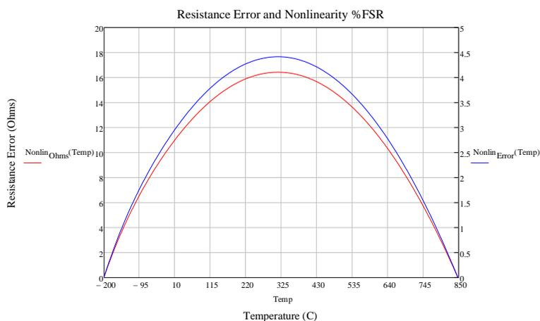
Figure 8. PT-100 RTD Non-Linearity from  $-200^{\circ}\text{C}$  to  $850^{\circ}\text{C}$
