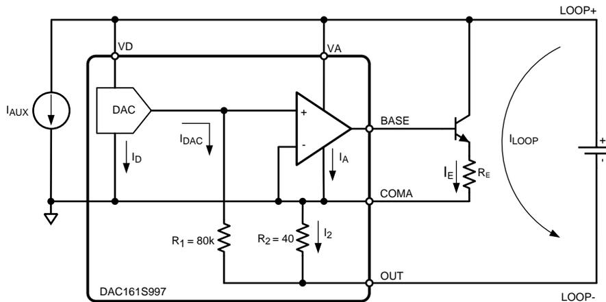
Figure 12. Loop-Powered Transmitter
