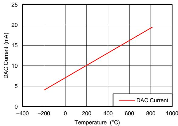
Figure 45. Ideal DAC Loop Current vs Temperature Range
