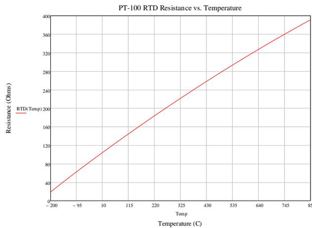
Figure 7. PT-100 RTD Resistance from  $-200^{\circ}\text{C}$  to  $850^{\circ}\text{C}$
