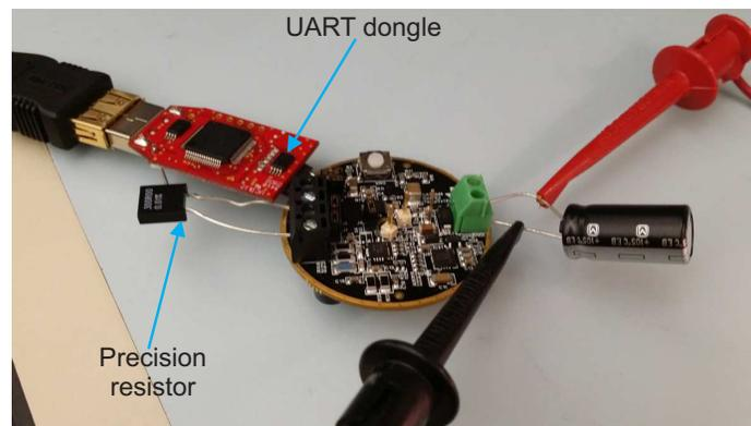
**Figure 24. System Hardware Setup for MSP430 Firmware programming**
