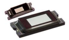
Figure 3-2. A 0.2" Diagonal DMD (e.g. DLP2010) Compared to a 0.45" Diagonal DMD (e.g. DLP4501)
