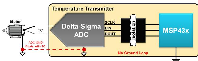
Figure 1. Breaking Ground Loops with Digital Isolation
