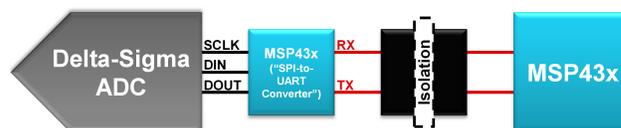
Figure 4. Isolation Scheme Using "SPI-to-UART Converter"
