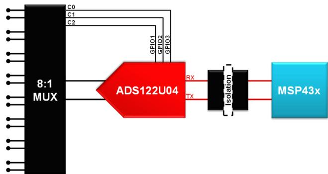
Figure 7. Controlling External MUX with GPIO Pins on ADS122U04
