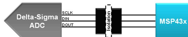
Figure 3. Isolation Scheme Using 3-wire SPI
