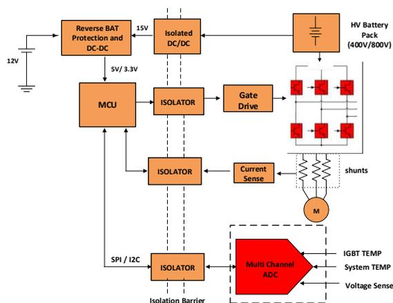
**Figure 1. Typical HV Traction Inverter**
