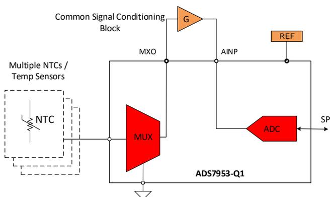
**Figure 3. Typical Block Diagram Showing Multiple NTCs Interfaced with ADS7953-Q1**
