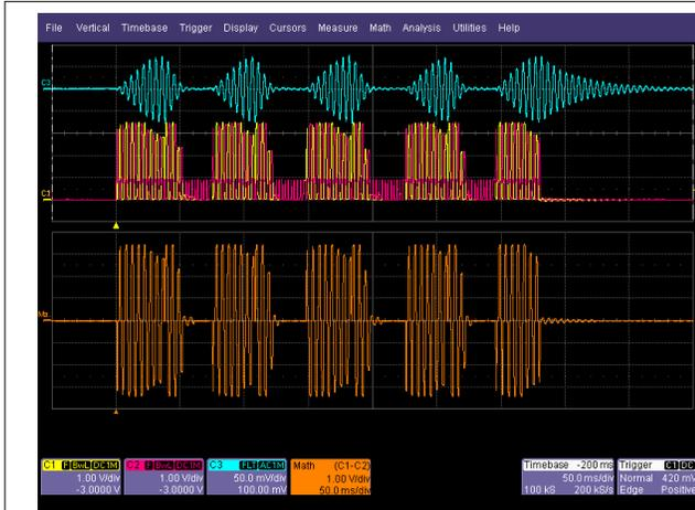
**Figure 2-5. LRA Pulsing Waveform**
