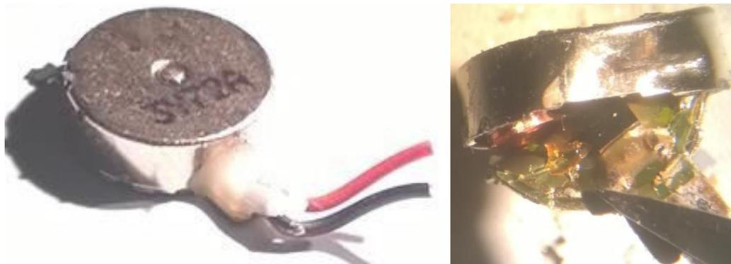
**Figure 2-3. BLDC Module Picture**
