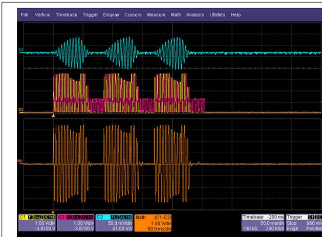
Figure 4-6. LRA Triple Click Waveform - AAC1030
