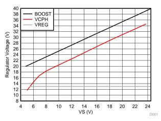
Figure 7. Regulator Voltage versus VS
