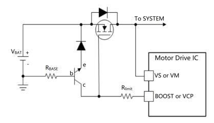
Figure 6. Reverse Battery Protection With Motor Drive IC
