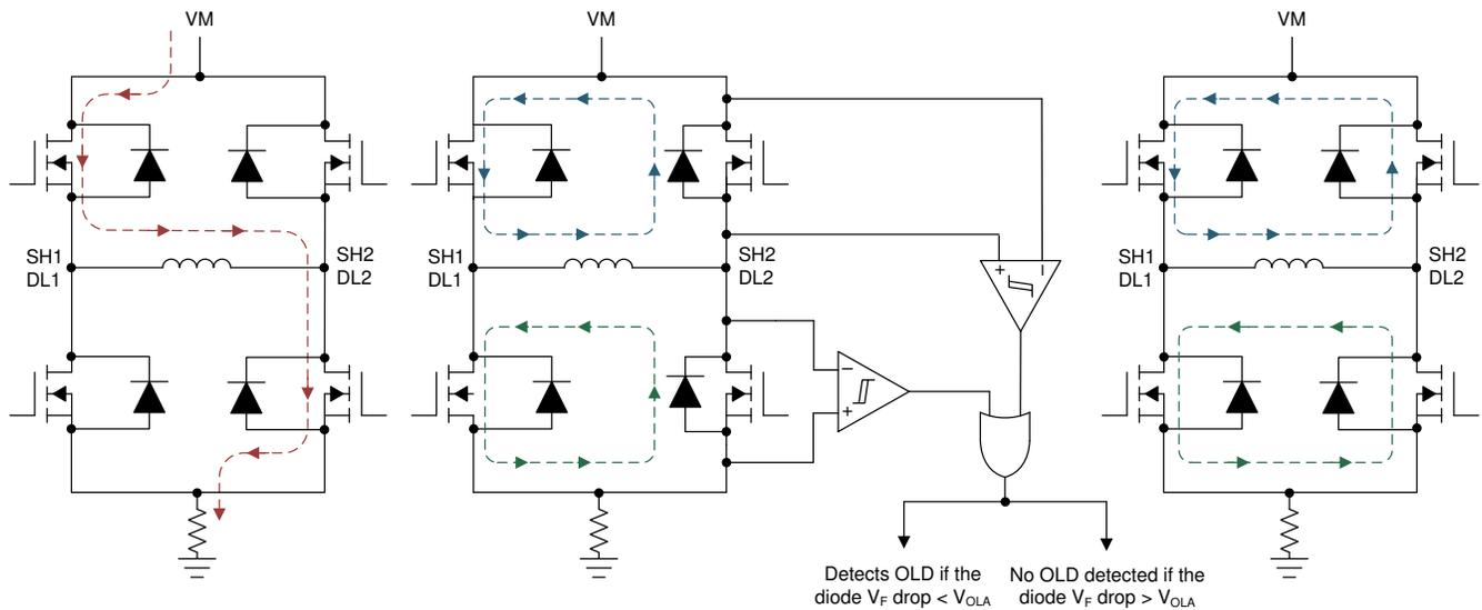
Figure 3-6. Circuit for Active OLD in a BLDC Gate Driver
