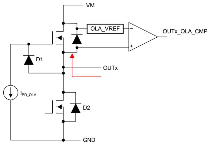
**Figure 3-5. Circuit for Active OLD in a DRV824x-Q1 device**
