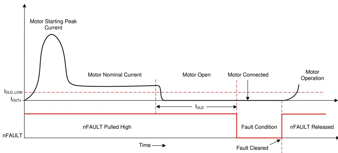
Figure 4-1. Low-Current Active OLD Operation
