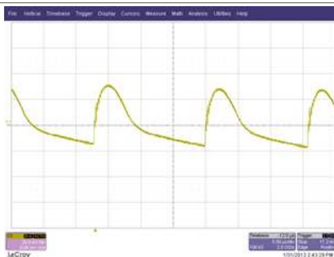
Figure 46. Ripple with 5-V, 1.2-A Output, 265- V_{AC} Input, 20 mV/div 5 \mu s/div
