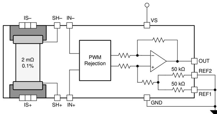
图 7-6. Ground-Referenced Output
