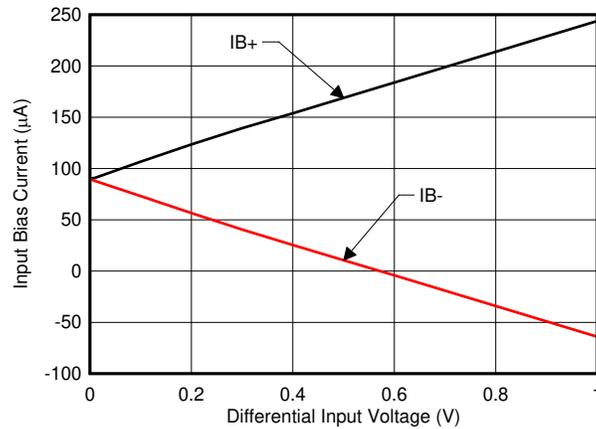
图 8-2. Input Bias Current vs Differential Input Voltage
