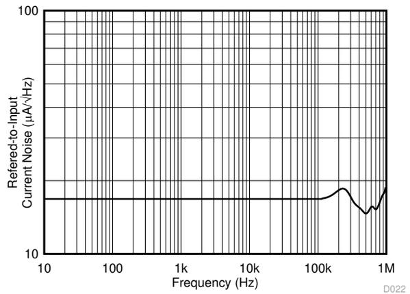
**图 6-22. INA253A3-Q1 Input-Referred Voltage Noise vs Frequency**
