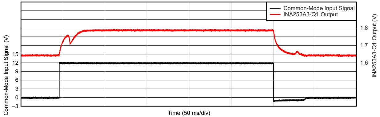
图 8-4. Solenoid Drive Current Sense Input and Output Signals
