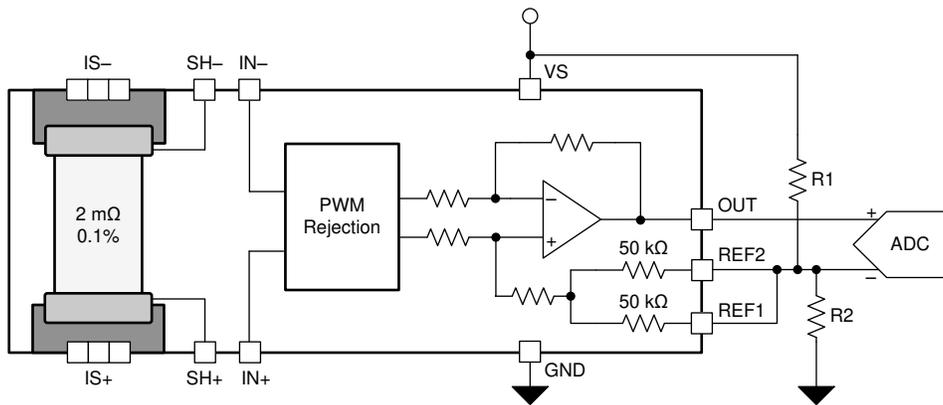
**图 7-10. Setting the Reference Using a Resistor Divider**
