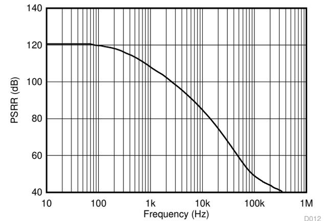
图 6-12. Power-Supply Rejection Ratio vs Frequency
