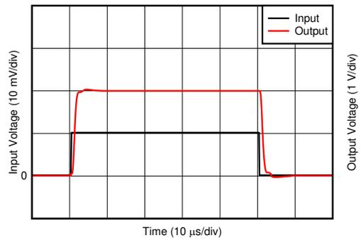
$V_{REF1} = V_{REF2} = 0$  V, 10-mV<sub>PP</sub> input step
