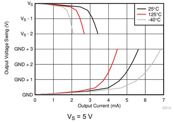
图 6-14. Output Voltage Swing vs Output Current
