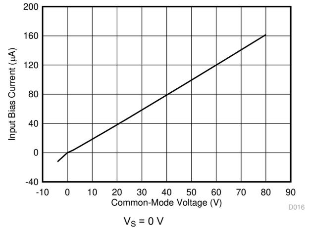
图 6-16. Input Bias Current vs Common-Mode Voltage
