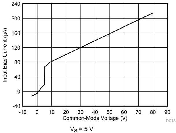
图 6-15. Input Bias Current vs Common-Mode Voltage
