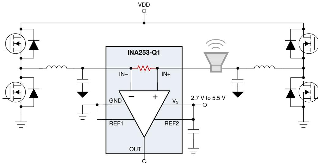
图 8-5. Current Sensing in a CLASS-D Subsystem
