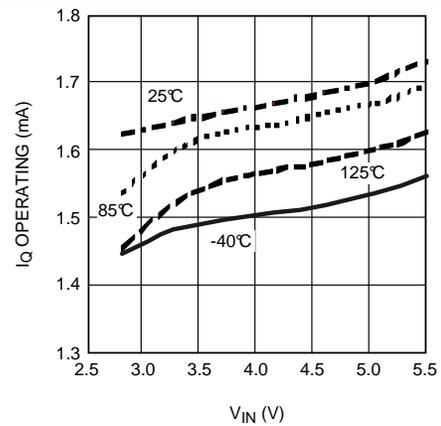
Figure 8.  $I_Q$  (operating) vs  $V_{IN}$  and Temperature
