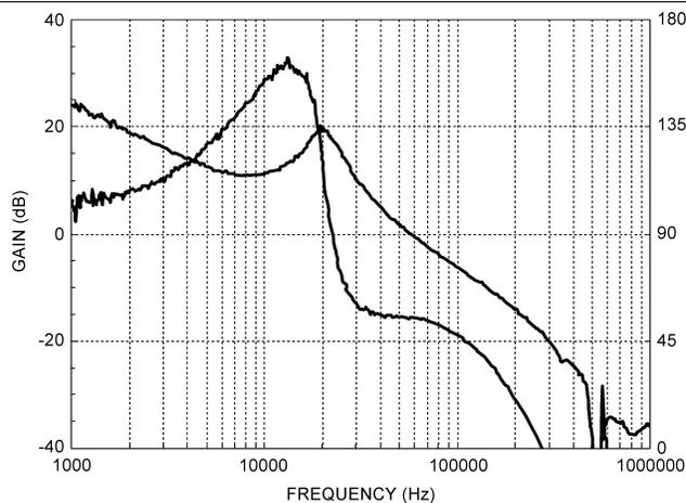
Figure 33. LM2854 500-kHz Bode Plot  $V_{IN} = 3.3\text{ V}$ ,  $V_{OUT} = 1.8\text{ V}$ ,  $I_{OUT} = 4\text{ A}$   $R_{FB1} = 250\text{ k}\Omega$ ,  $R_{COMP} = 1\text{ k}\Omega$ ,  $C_{COMP} = 47\text{ pF}$ ,  $L_{OUT} = 1.5\ \mu\text{H}$ ,  $C_{OUT} = 100\text{-}\mu\text{F}$  Ceramic
