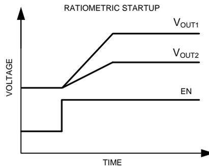
**Figure 17. Simplified Start-up Waveforms When Using Proportional Tracking**
