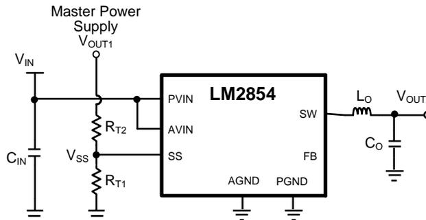
**Figure 14. Simplified Schematic Showing Use of Tracking**
