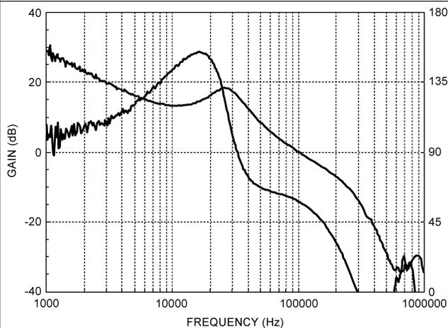
Figure 32. LM2854 1-MHz Bode Plot  $V_{IN} = 3.3\text{ V}$ ,  $V_{OUT} = 1.8\text{ V}$ ,  $I_{OUT} = 4\text{ A}$   $R_{FB1} = 150\text{ k}\Omega$ ,  $R_{COMP} = 1\text{ k}\Omega$ ,  $C_{COMP} = 100\text{ pF}$ ,  $L_{OUT} = 0.82\ \mu\text{H}$ ,  $C_{OUT} = 100\text{-}\mu\text{F}$  Ceramic
