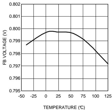
Figure 1. Feedback Voltage vs Temperature
