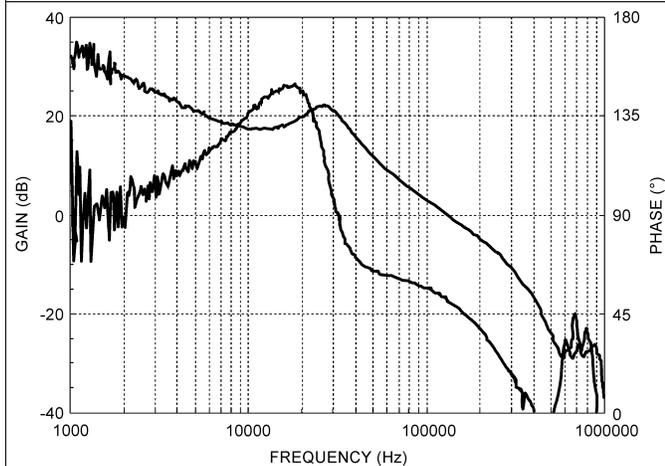
**Figure 36. LM2854 1-MHz Bode Plot  $V_{IN} = 5\text{ V}$ ,  $V_{OUT} = 3.3\text{ V}$ ,  $I_{OUT} = 4\text{ A}$   $R_{FB1} = 150\text{ k}\Omega$ ,  $R_{COMP} = 1\text{ k}\Omega$ ,  $C_{COMP} = 68\text{ pF}$ ,  $L_{OUT} = 0.82\text{ }\mu\text{H}$ ,  $C_{OUT} = 100\text{-}\mu\text{F Ceramic}$**
