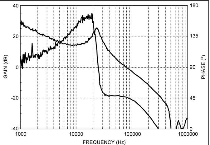
**Figure 37. LM2854 500-kHz Bode Plot  $V_{IN} = 5\text{ V}$ ,  $V_{OUT} = 3.3\text{ V}$ ,  $I_{OUT} = 4\text{ A}$   $R_{FB1} = 250\text{ k}\Omega$ ,  $R_{COMP} = 1\text{ k}\Omega$ ,  $C_{COMP} = 33\text{ pF}$ ,  $L_{OUT} = 1.5\text{ }\mu\text{H}$ ,  $C_{OUT} = 100\text{-}\mu\text{F Ceramic}$**
