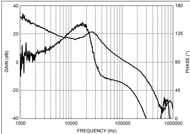
**Figure 34. LM2854 1-MHz Bode Plot  $V_{IN} = 5\text{ V}$ ,  $V_{OUT} = 1.8\text{ V}$ ,  $I_{OUT} = 4\text{ A}$   $R_{FB1} = 150\text{ k}\Omega$ ,  $R_{COMP} = 1\text{ k}\Omega$ ,  $C_{COMP} = 100\text{ pF}$ ,  $L_{OUT} = 0.82\text{ }\mu\text{H}$ ,  $C_{OUT} = 100\text{ }\mu\text{F}$**
