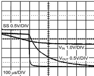
Figure 40. LM2854 500-kHz Power Off Characteristic
