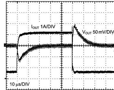
Figure 41. LM2854 1-MHz Load Transient Response
