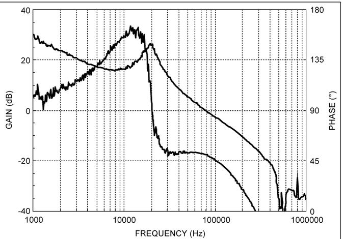
**Figure 35. LM2854 500-kHz Bode Plot  $V_{IN} = 5\text{ V}$ ,  $V_{OUT} = 1.8\text{ V}$ ,  $I_{OUT} = 4\text{ A}$   $R_{FB1} = 250\text{ k}\Omega$ ,  $R_{COMP} = 1\text{ k}\Omega$ ,  $C_{COMP} = 47\text{ pF}$ ,  $L_{OUT} = 1.5\text{ }\mu\text{H}$ ,  $C_{OUT} = 100\text{-}\mu\text{F Ceramic}$**
