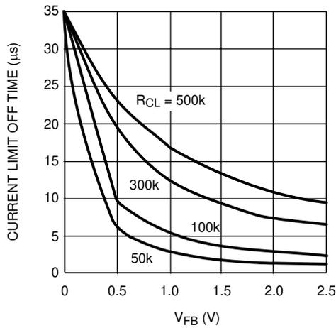
图 6-3. Current Limit Off-Time vs  $V_{FB}$  and  $R_{CL}$
