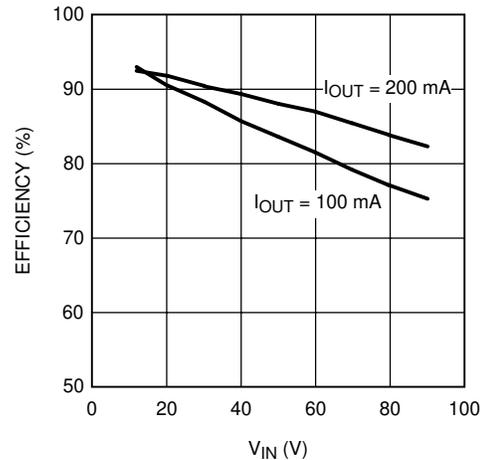
图 8-3. Efficiency vs  $V_{IN}$  and Load Current
