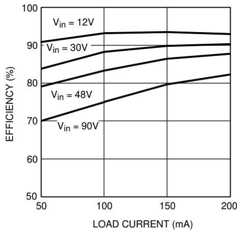
图 8-2. Efficiency vs Load Current and  $V_{IN}$
