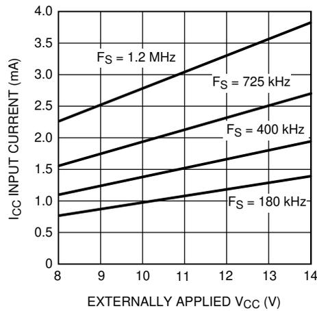
图 6-5.  $I_{CC}$  Current vs Applied  $V_{CC}$  Voltage
