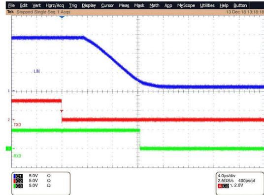
图 10-12. Recessive to Dominant Propagation Delay
