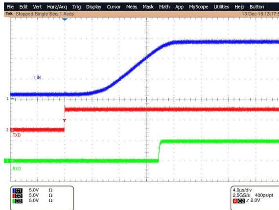
图 10-13. Dominant to Recessive Propagation Delay
